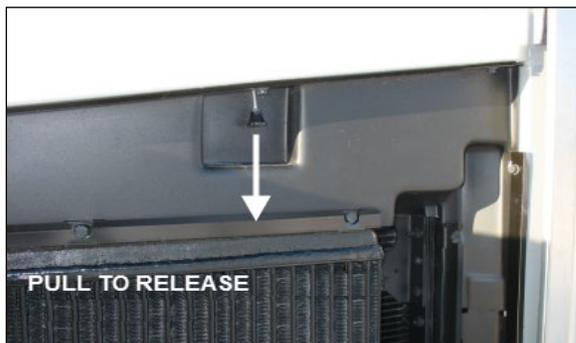
**UNLOCKING SCR CONVERTER ACCESS DOOR**
