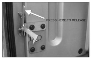
EVAPORATOR COMPARTMENT DOOR SECONDARY LOCK LEVER
