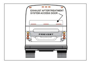
The engine door must be open before opening the exhaust aftertreatment system access door. To open the access door, lower the latch release lever, using a flat tip screwdriver.
