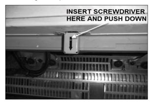
To close the door, lower the door and push against the release lever spring to latch the door shut.
