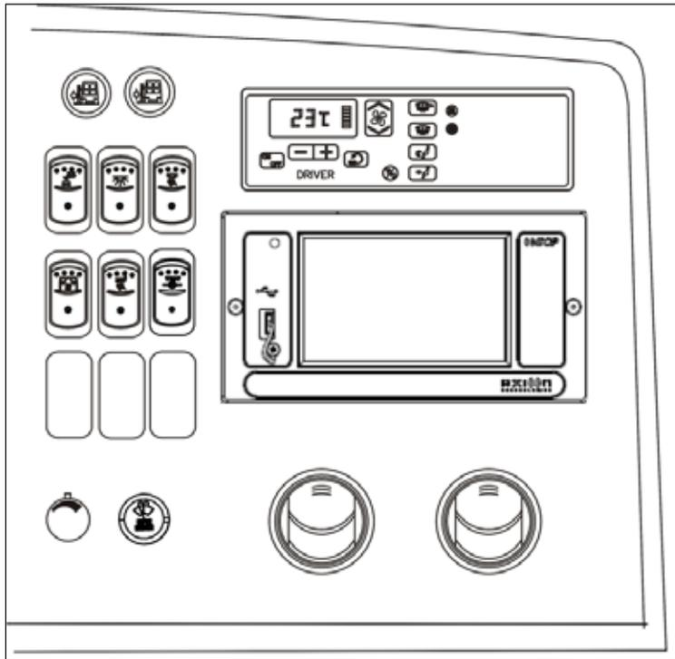
The HVAC control module, electronic destination sign control unit as well as the cluster dimmer switch, interior lighting control switches, entrance door operating buttons, miscellaneous door operating buttons, miscellaneous control switches and air vents are located on the R.H. dashboard panel.
