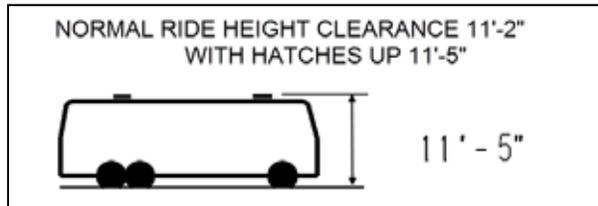
Vehicle height information with hatches up and down.
