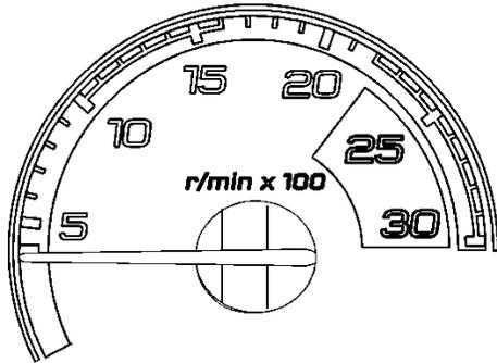
**Tachometer (rpm x 100)**
