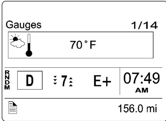
The outside air temperature, fuel flow and the odometer (Allison transmission) are part of the default display. You can replace the default display by your selection of favorite gauges using the Driver Information Display sub-menu Favorite Display Setting. Refer to *Other Features* section for more information.
