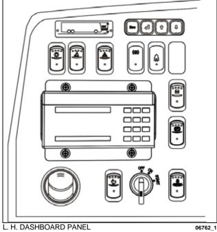
The L.H. dashboard panel includes controls for the operation of the coach; it also includes the ignition switch, radio control and an adjustable air vent.
