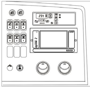
The HVAC control module, electronic destination sign control unit as well as the cluster dimmer switch, interior lighting control switches, entrance door operating buttons, miscellaneous control switches and air vents are located on the R.H. dashboard panel.
