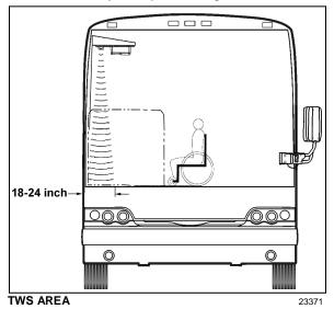
3. Turn sensor angle adjustment screw clockwise to move direction of beam away from center aisle and towards doorway. Stop adjustment when LED ceases to flash.
