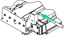
3. Turn the manual platform release shafts using pump handle extension to disengage the platform and then lift the stowlock mechanical catch.
