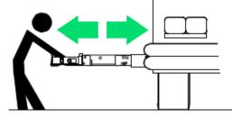
Turn the manual platform release shafts 5. using pump handle extension back to previous position to lock the platform.
