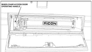
OPENING LIFT MECHANISM ACCESS DOOR 18616
