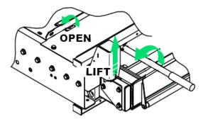
4. Grasp the platform and pull firmly until the lift is all the way out against the carriage stops.
