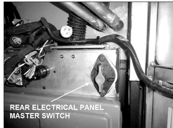
REAR ELECTRICAL PANEL IN R.H. ENGINE COMPARTMENT
