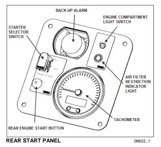
3. Press the *REAR START* pushbutton switch, release push-button after the engine starts.
