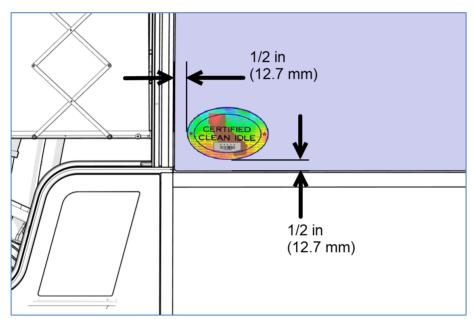
Figure 4: CLEAN IDLE LABEL POSITION ON X3 SERIES
