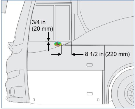
Figure 5: CLEAN IDLE LABEL POSITION ON VOLVO 9700
