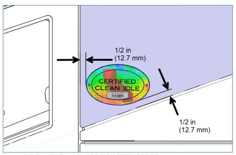
Figure 3: CLEAN IDLE LABEL POSITION ON **H3 SERIES**
