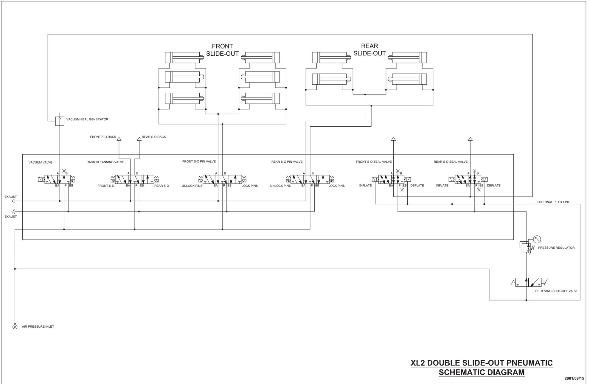
**XL2 DOUBLE SLIDE-OUT PNEUMATIC SCHEMATIC DIAGRAM**
