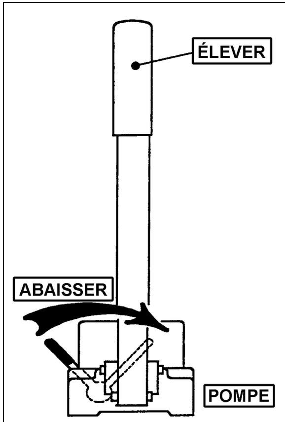
FONCTIONNEMENT MANUEL DU SYSTÈME D'ÉLEVATION 23283F
