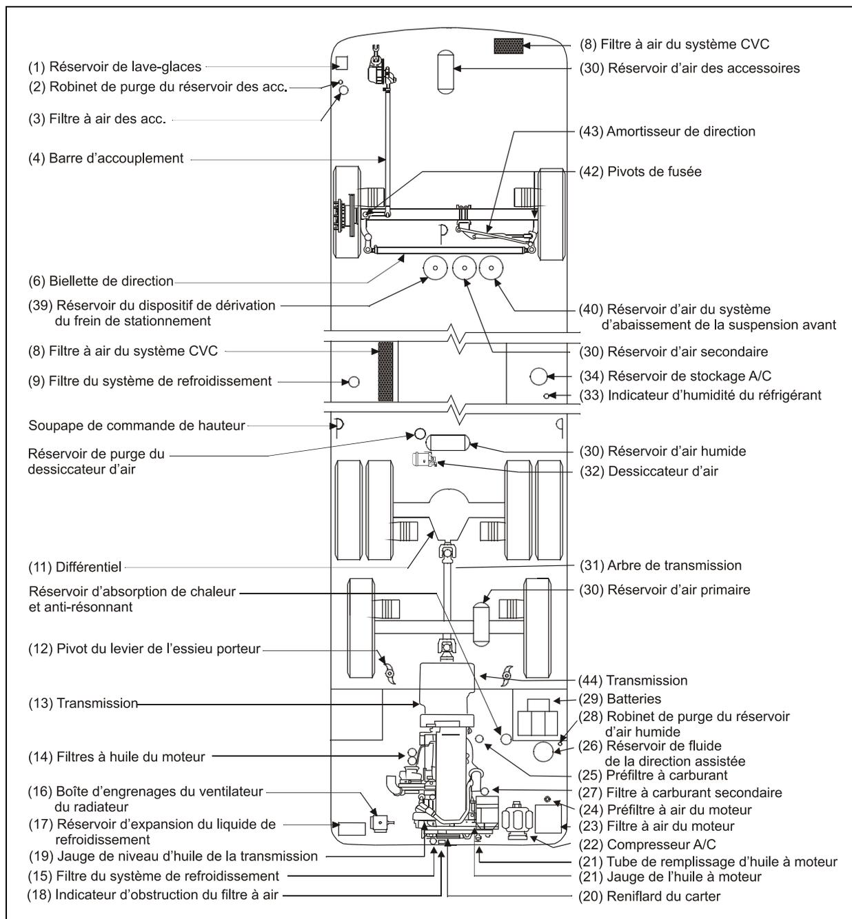
POINTS DE LUBRIFICATION ET D'ENTRETIEN POUR UN VÉHICULE AVEC SUSPENSION RIGIDE (TYPIQUE)
