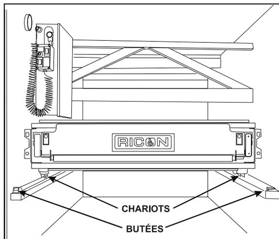
FONCTIONNEMENT MANUEL DU SYSTÈME D'ÉLEVATION
