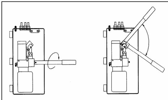
ÉLÉVATION DE LA PLATE-FORME DE FAÇON MANUELLE
