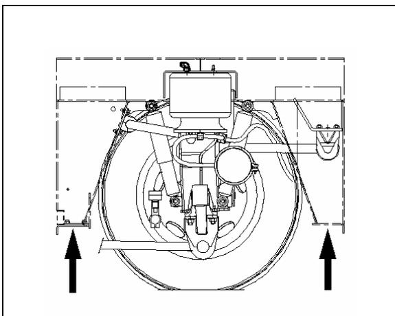
POINT DE LEVAGE SOUS LE CHÂSSIS AVANT -
