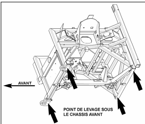
POINT DE LEVAGE SOUS LE CHÂSSIS AVANT -
