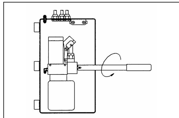
ABAISSEMENT DE LA PLATE-FORME DE FAÇON MANUELLE
