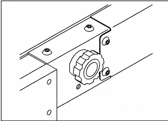
**BOUCHON DE COMMANDE MANUELLE DE LA BUTÉE ESCAMOTABLE**
