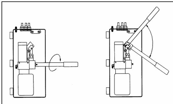
ÉLÉVATION DE LA PLATE-FORME DE FAÇON MANUELLE
