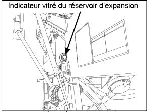
INDICATEUR VITRÉ DU RÉSERVOIR D'EXPANSION, COMPARTIMENT MOTEUR
