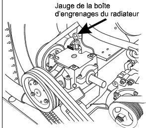
JAUGE DE LA BOÎTE D'ENGRENAGES DU RADIATEUR, COMPARTIMENT MOTEUR
