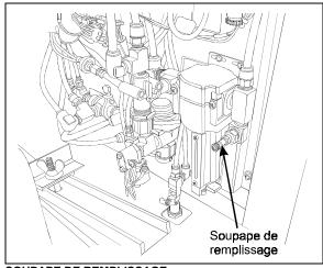
SOUPAPE DE REMPLISSAGE, COMPARTIMENT DE SERVICE AVANT
