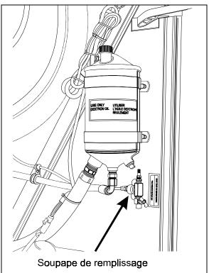
SOUPAPE DE REMPLISSAGE, COMPARTIMENT MOTEUR (CÔTÉ DROIT)
