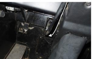
Route the harness inside the front junction box up to the lateral control panel area (use cable ties as required to secure the harness inside the junction box).
