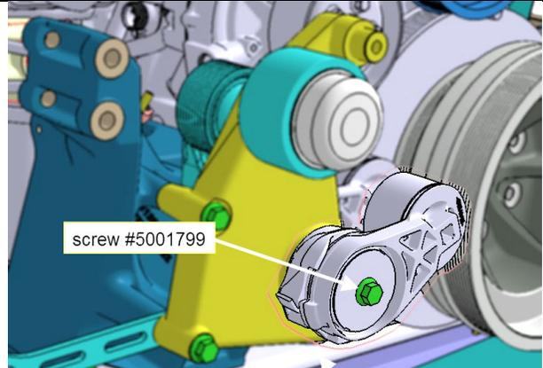
**FIGURE 66: TENSIONER MOUNTING SCREW TORQUE : 48 lb-ft**
