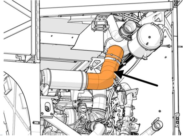
**FIGURE 105: REINSTALL THIS EXHAUST PIPE SECTION**
