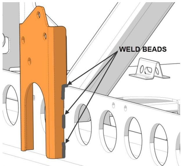
65. As a preparation for **welding**, use a grinder with abrasive disc to remove some paint to reach bare metal. Weld the **ground stud** #380360 centered on the beam, at 16 inches (406 mm) from the vertical member beam end.
