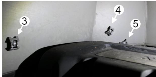
FIGURE 112: TIE MOUNT 3 & 4 SHALL NOT BE PLACED BETWEEN THE BULKHEAD AND THE VALVE COVER.
