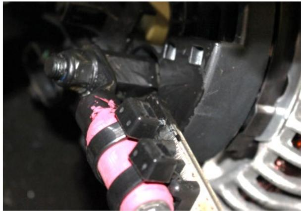
**FIGURE 136: POSITIVE (+) CONNECTION ON THE ALTERNATOR**
