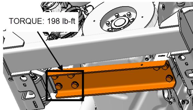
FIGURE 55: FOUR (4) SCREWS UNDER THE REINFORCEMENT CHANNEL
