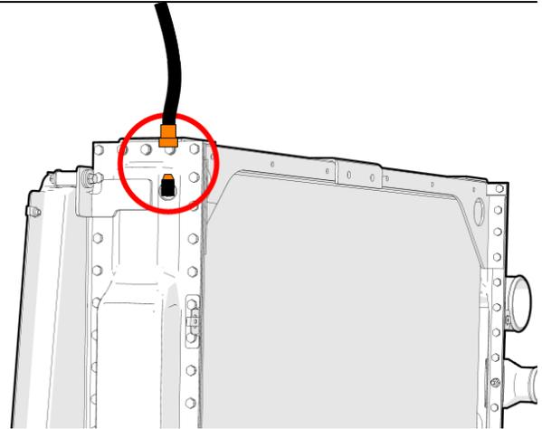
13. Disconnect **electrical connector** from the fan clutch. The remaining connector on the chassis cable will be capped and left in place.
