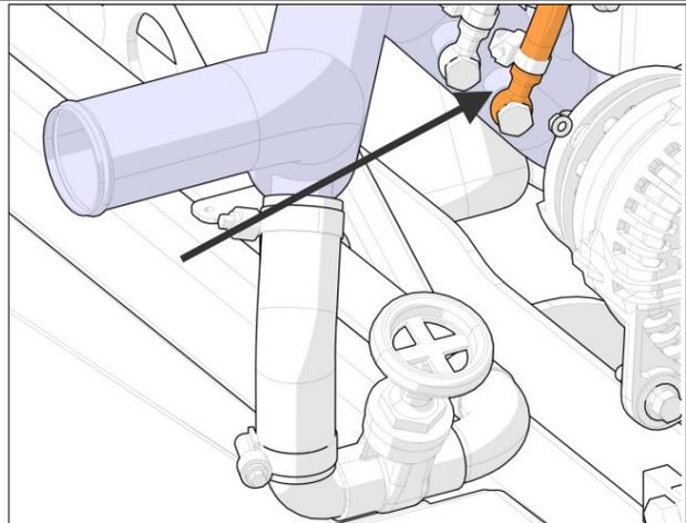
FIGURE 93: DEF INJECTOR COOLANT LINE RETURN HOSE
