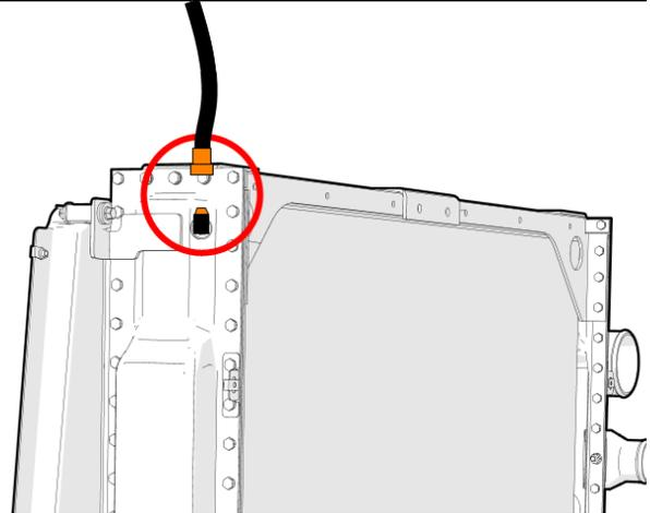
116. Reinstall the cooling pack protector tube with the following hardware:
