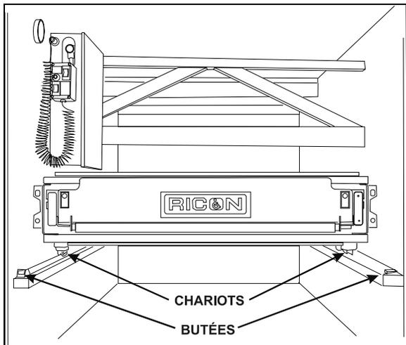
FONCTIONNEMENT MANUEL DU SYSTÈME D'ÉLÉVATION
