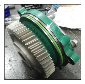
10. Slide the new PTO in place (pry coolant hose as required). Make sure the O-ring is engaging smoothly.
