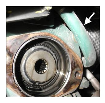
8. Clean the PTO mounting surfaces (make sure debris are not falling inside the engine).
