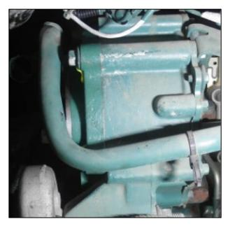
12. Clean the hydraulic pump mounting surface & install the new supplied # **925259** hydraulic pump O-Ring (slightly oil the O-ring).
