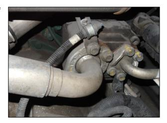
6. Remove the pump from the vehicle (discard pump O-ring).
