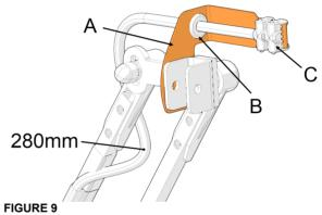
A= nozzle assembly support bracket B= grommet C= nozzle assembly
