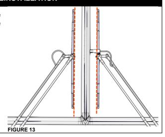
21. Tighten the wiper arms nut to **22 lbs-ft**. Reinstall the caps from the pivots.
