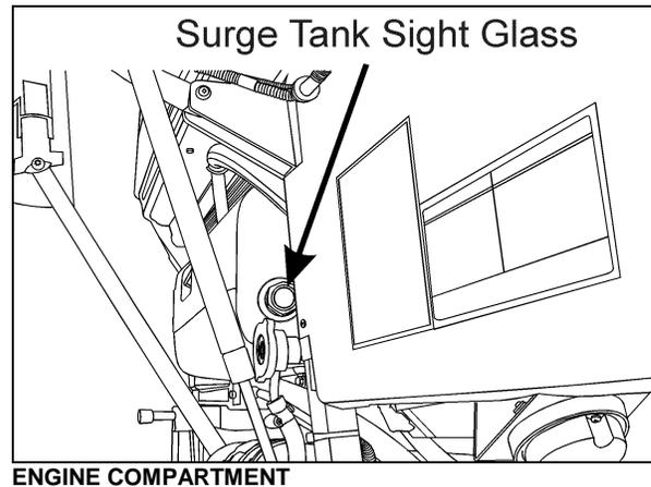
**Warning :** Hot engine coolant is under high pressure. Allow engine to cool down before adding coolant.
