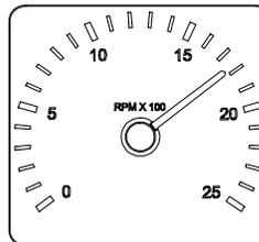
Indicates the operating speed of the engine in hundreds of revolutions per minute (rpm x 100). The tachometer serves as a guide for gear shifting and helps to prevent engine over-speeding when driving downhill with the JACOBS engine brake operating. The maximum allowable engine speed is 2,450 rpm.
