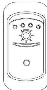
Push down rocker switch to the first position to activate clearance, tail and marker lights. Push down fully to turn ON both the clearance and marker lights and the headlights. The controls and instrument lights will illuminate.
