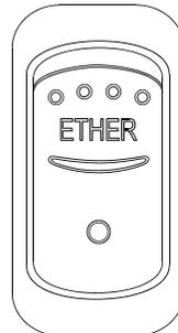
Activates the engine cold starting aid. Refer to "Starting and Stopping Procedures" chapter 5.
