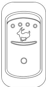
For extended idling periods, run the engine at fast idle. Press down the rocker switch to engage fast idle. This increases the engine speed to approximately 1,000 rpm.
