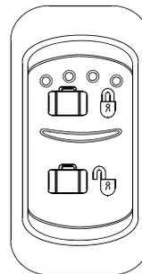
This optional system enables locking all baggage compartment doors by pressing down on the upper portion of the switch. To unlock all compartments, press down on the lower portion of the switch.
