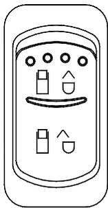
Use this rocker switch located on the dashboard's R.H. side panel for locking or unlocking the entrance door from the inside.
