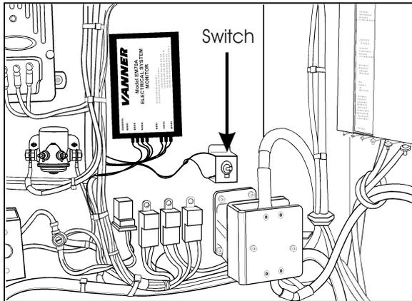
MASTER SWITCH IN MAIN POWER COMPARTMENT
