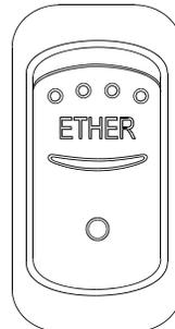
Activates the engine cold starting aid. Refer to "Starting and Stopping Procedures" chapter 5.
