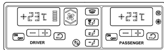
Separate driver and cabin heating, ventilation and air conditioning controls are located on this panel. To operate, the motorcoach's engine must be running.
