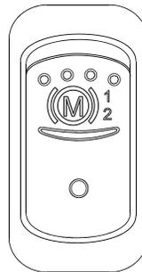
Press down rocker switch to the first position to actuate system to 2/3 engine brake and press to the second position for a full application of engine brake. Refer to "Other Features" chapter 4.
