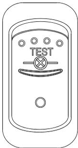
Press this switch while ignition is in the *ON* position to illuminate the telltale light cluster. Perform this test to verify indicator light functionality. Telltale lights will extinguish automatically after about ten seconds.
