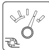
Indicates turbo boost pressure in psi. Reading depends on engine rpm and load conditions.
