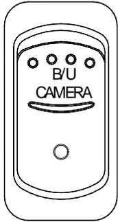
Press down this switch to turn *ON* the Back-Up Camera's monitor when the transmission of the motorcoach is not in the reverse gear.
