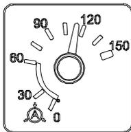
Indicates the accessories air system pressure. The normal operating pressure is from 95 to 125 psi (655 to 860 kPa).
