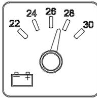
Indicates the condition of the 24-volt electrical system. With the engine running, the normal reading should be between 26.5 and 28.0 volts.
