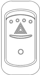
Depress the rocker switch to make all turn signal lights flash at once. The dashboard telltale lights will flash when the hazard warning flashers are ON.
