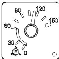
Indicates the primary air system pressure. The normal operating pressure is from 95 to 125 psi (655 to 860 kPa).
