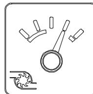
Indicates turbo boost pressure in psi. Reading depends on engine
