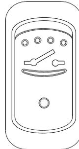
Both the 12-volt and 24-volt systems are activated by the master switch located on the L.H. lower control panel. A telltale light on the L.H. dashboard will illuminate when the ignition key is in the OFF position.
