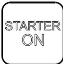
Illuminates when the engine starter is on.
