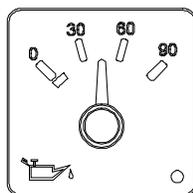
Indicates engine oil pressure. The normal reading should be between 50 and 70 psi (345 - 480 kPa) at 55 mph (90 km/h). A low oil pressure indicator LED (bottom right corner) illuminates when the oil pressure drops below 50 psi (345 kPa).
