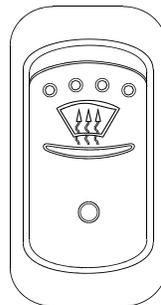
Depress this switch to the first position to operate the defogger blower at low speed, press down fully to operate the blower at high speed.
