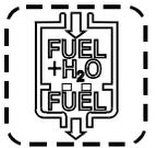
Illuminates when accumulated water in the fuel filter/water separator needs to be drained. Refer to "Care and Maintenance" chapter 7.
