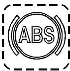
Illuminates when the ABS is not available or when the ABS is malfunctioning. Since the ABS system does not operate under 4 mph (7 km/h), the indicator will remain illuminated until the coach reaches that speed. Refer to "Other Features" chapter 4.
