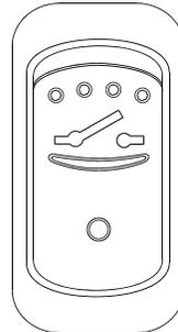
Both the 12-volt and 24-volt systems are activated by the master switch located on the L.H. lower control panel. A telltale light on the L.H. dashboard will illuminate when the ignition key is in the *OFF* position.
