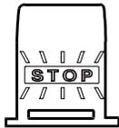
Illuminates when rear stop lights illuminate. This occurs when either cruise control DECEL switch, service brakes, parking brakes, engine retarder or transmission retarder is applied.
