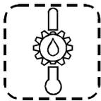
Illuminates when the transmission oil temperature is too high. Disengage the retarder to allow the oil temperature to cool down.
