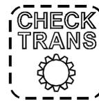
Illuminates briefly when the ignition is switched ON as a light test. The indicator light should go out after two seconds.
