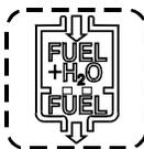
Illuminates when accumulated water in the fuel filter/water separator needs to be drained. Refer to "Care and Maintenance" chapter 7.
