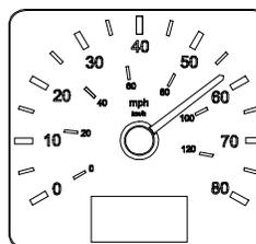
Indicates the motorcoach speed in miles per hour (mph) and kilometers per hour (km/h).
