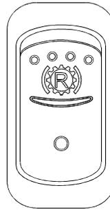
Press down rocker switch to actuate transmission retarder. Refer to "Steering Column Controls" in this chapter.
