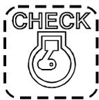
Illuminates when the ignition switch is ON as a light bulb check. The light should turn OFF after five seconds. If the indicator remains ON after five seconds or comes ON sometime after starting the engine, the Detroit Diesel Electronic Control (DDEC) system has detected a minor problem.
