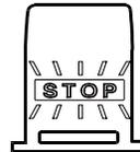
Illuminates when rear stop lights illuminate. This occurs when either cruise control DECEL switch, service brakes, parking brakes, engine retarder or transmission retarder is applied.
