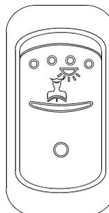
Press down the rocker switch to illuminate the ceiling lights in the driver's area as needed.
