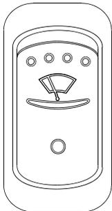
Depress the wiper rocker switch to the first position for intermittent wiping. For continuous wiping, depress switch fully.
