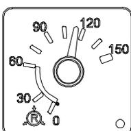
Indicates the secondary air system pressure. The normal operating pressure is from 95 to 125 psi (655 to 860 kPa).
