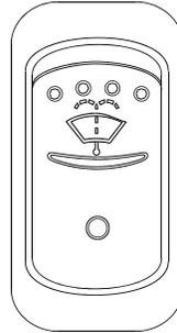
Hold down rocker switch to spray windshield washer fluid.
