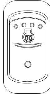
Push down rocker switch to turn the coolant heating system ON, supplementing the central heating system when required. The coolant heater will turn ON or OFF automatically depending on coolant temperature.
