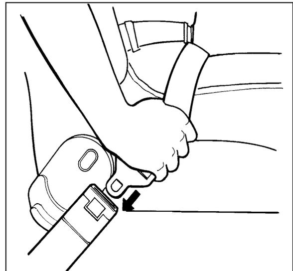
**Note :** The safety belt must be pulled out slowly and continuously, otherwise it will lock the reel before the latch plate reaches the buckle. If this happens, allow the belt to retract completely and repeat the procedure correctly.
