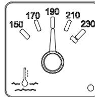
Indicates the operating temperature of the engine coolant. The normal reading should be between 190°F and 215°F (88°C to 102°C).
