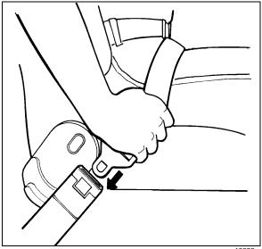
Note: The safety belt must be pulled out slowly and continuously, otherwise it will lock the reel before the latch plate reaches the buckle. If this happens, allow the belt to retract completely and repeat the procedure correctly.
