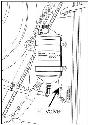
FILL VALVE IN ENGINE COMPARTMENT
