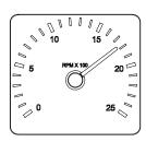
Indicates the operating speed of the engine in hundreds of revolutions per minute (rpm x 100). The tachometer serves as a guide for gear shifting and helps to prevent engine over-
