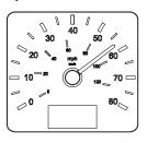
Indicates the motorcoach speed in miles per hour (mph) and kilometers per hour (km/h).
