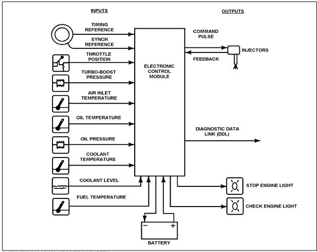
SHEMATIC DIAGRAM OF DDEC IV SYSTEM
