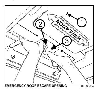
**Note:** In the event of ventilation blower motor failure, the emergency roof escape may be used to aid ventilation by pushing the hatch upward.
