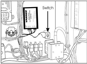
MASTER SWITCH IN MAIN POWER COMPARTMENT
