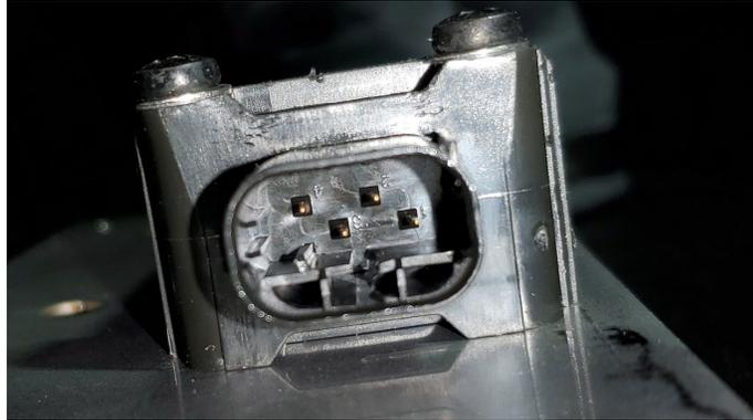
6. Make sure that the connector is the appropriate one. Inappropriate connector will not lock properly and may not be watertight.
