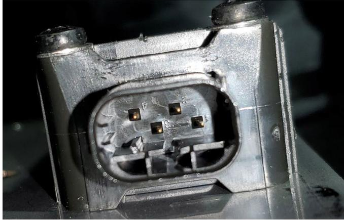
8. Make sure that the connector is the appropriate one. Inappropriate connector will not lock properly and may not be watertight.
