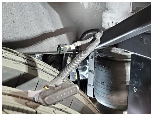
5. Check inside the antennas connector and make sure that the connector pins are in proper condition.
