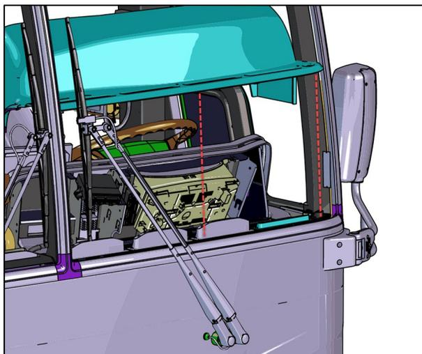
2. Disconnect and remove the existing TPMS module.
