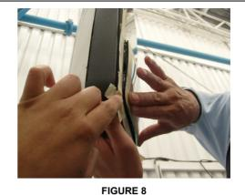
9. Carefully remove the excess of **Sika® 271.** Carefully remove the masking tape from mirrors.
