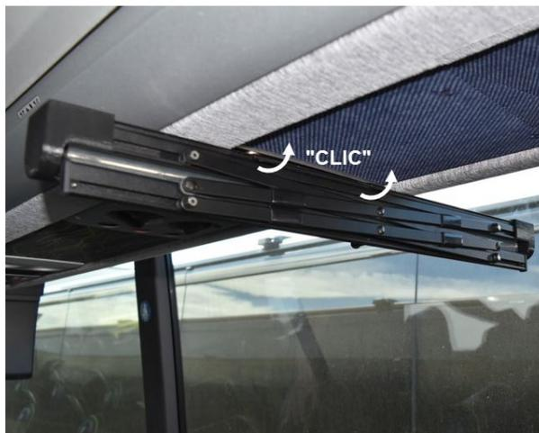
7. Put back the overhead console to finish the installation.
