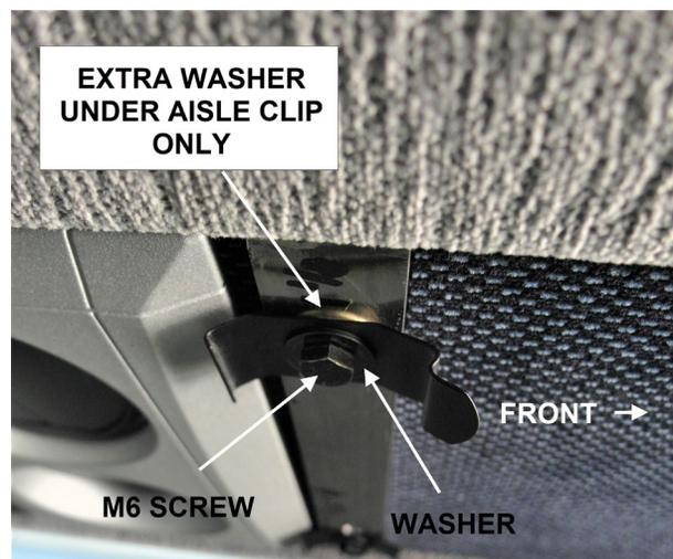
6. Clip in place the scissor screen and check for correct adjustment. The screen should deploy and retract easily and should not contact the side window or lateral sun shade. Adjust laterally as required.
