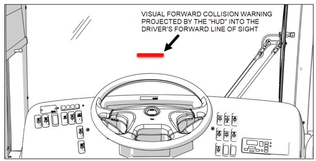
FIGURE 2: HEAD-UP DISPLAY PROJECTED VISUAL WARNING
