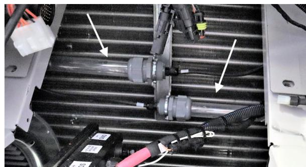
19. Insert the gray **FLUO L1** (top/left) & **FLUO R4** (bottom/right) connectors through the side holes of the housing to connect the fluo tubes.
