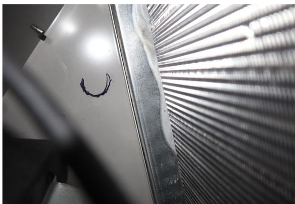
14. From the inside, drill a small pilot hole in the middle of the marks (both sides).
