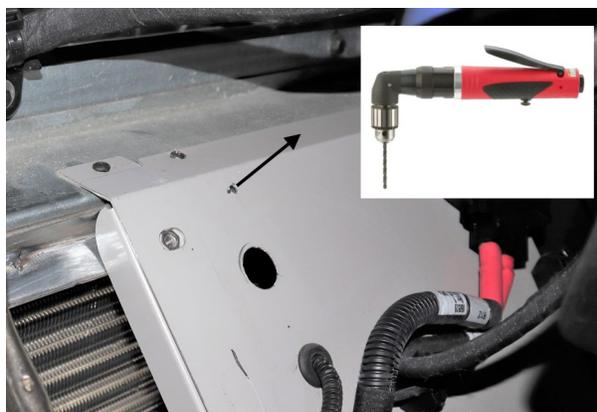
9. Secure the support using the supplied screws, washers & nuts.
