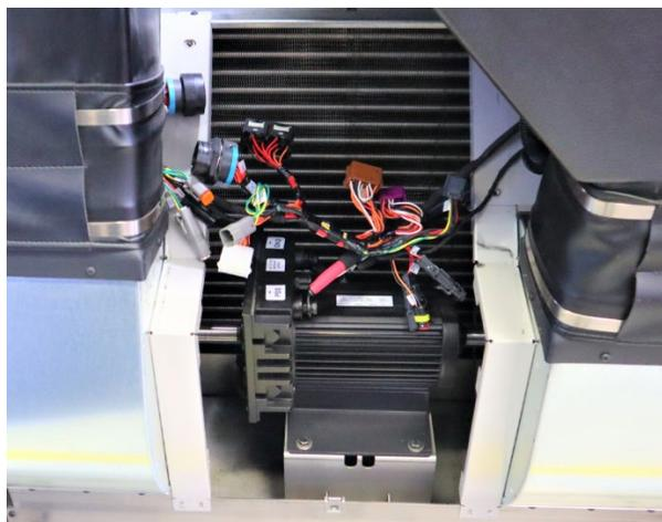
4. Two **7/8in** holes must be drilled behind the evaporator housing ducts (one on each side) to allow passage for the tubes power cables.
