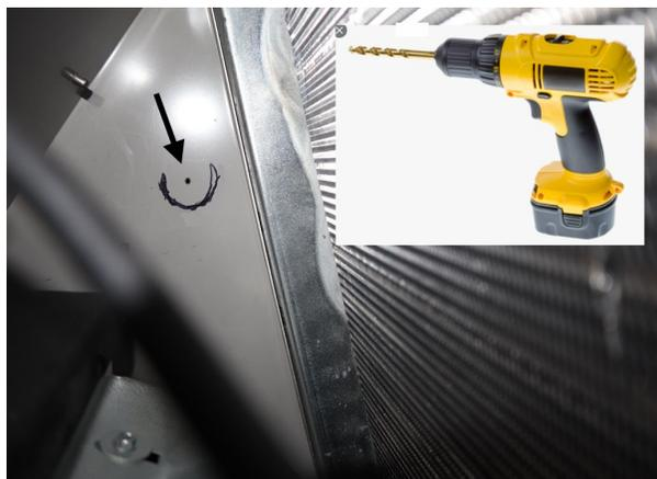
15. Before drilling the final (larger) holes, validate from the outside of the housing that the pilot holes are drilled at the correct positions.
