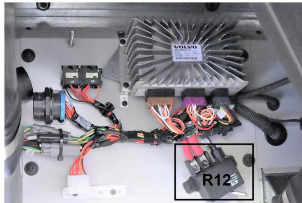
– Connect the **CB3 fused wire (10 amps)** of the ballast box to the **CB3 connection** of the **R12 relay** (left wire).
