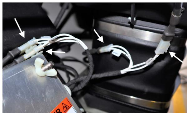
27. Fit the fully connected ballast box to the black plastic cover that goes over the I/O-EB module.
