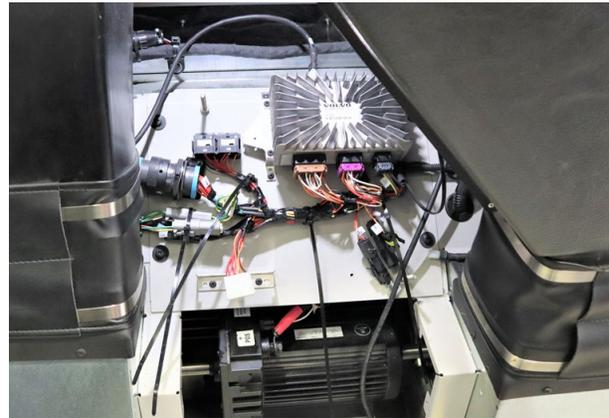
24. Reconnect the module, relays and surrounding harnesses. Also secure the harnesses with new **N91098** UV resistant cable ties.
