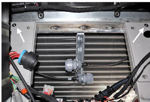
10. Remove the (plastic gray) tube hold-down nuts from all harnesses (UV1-A, UV1-B, UV2-A & UV2-B). Slide the hold-down nuts over the two tubes.
