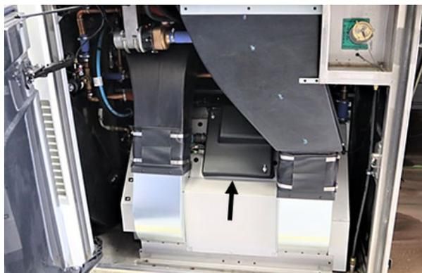
2. Disconnect the I/O-EB module. Also disconnect all harness connections and cable ties that prevent the removal of the upper cover (on which is mounted the I/O-EB module).
