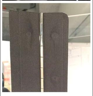
To protect the driver's hand, install the 509558 rubber molding strip on the lower edge of the door hinge (driver's armrest area).
