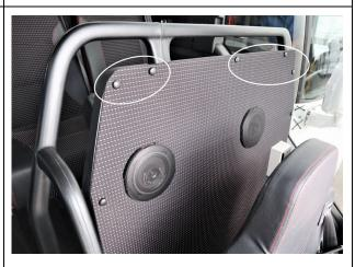
Also remove the two screws holding the panel on the aisle side (also keep black plastic caps but discard screws and plastic washers).
