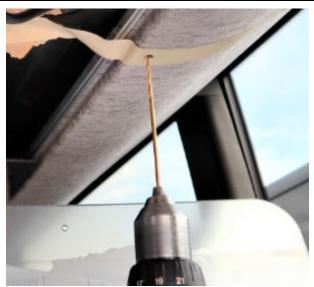
Secure the top support to the parcel rack using the supplied 500879 screws & 500464 washers.
