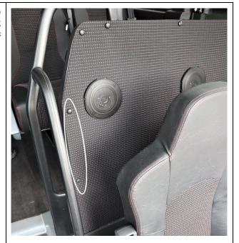
Behind the panel, unscrew halfway the two hex bolts holding the top of the handrail.
