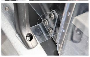
Secure (hand tight) the 45deg. support to the door hinge using a 502626 screw, one 5001182 nut & one 502571 rubberized washer (one of the upper hinge hole is drilled larger for this purpose).
