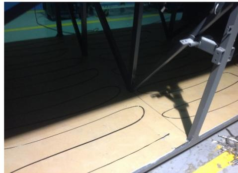
21. Install the central floor plates 21276271 and 21276269 and hold them with C-pliers on the edge.
