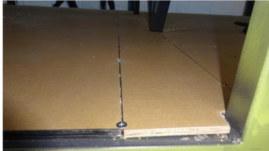
13. Mix the sealant and catalyst 8715036, and then apply it on the wood imperfections in order to have a flat surface.
