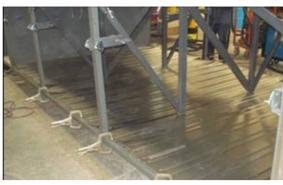
23. Install the central floor plates 21300395 and 21276269 and hold them with C-pilers on the edge.
