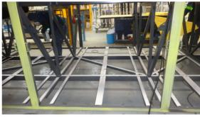
10. Apply sealant 8714628 on the perimeter of the luggage compartment profiles.
