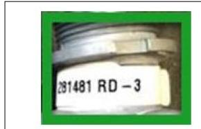
Figure 1: SPRING RETURN RD-3 TYPE VALVE LABEL – EMERGENCY/PARKING BRAKE OVERRULE VALVE
