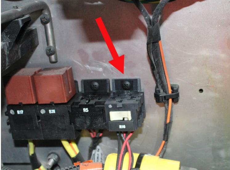
FIGURE 28: RELAY BASE & R16 ONCE INSTALLED
