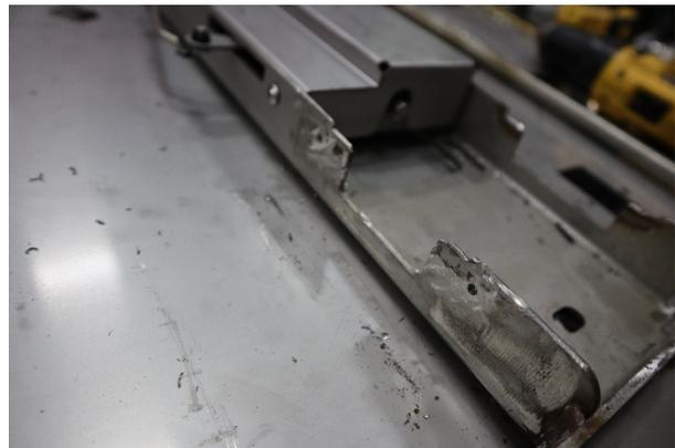
11. Enlarge the 3 holes enough to accept the 3 mounting screws supplied in the kit.
