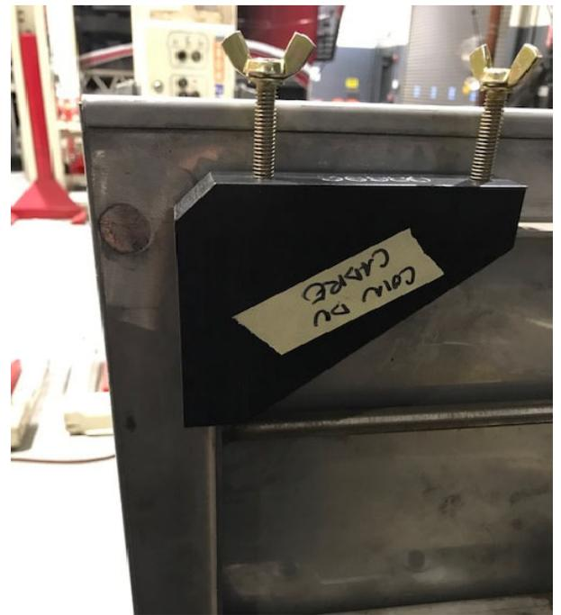
29. Mark the two drill points on the door frame (do not drill yet)
