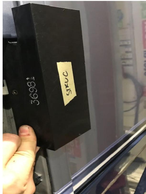
26. Position the new **2810362** upper door support bracket and secure to the vehicle using the supplied **9419967** metal screws.
