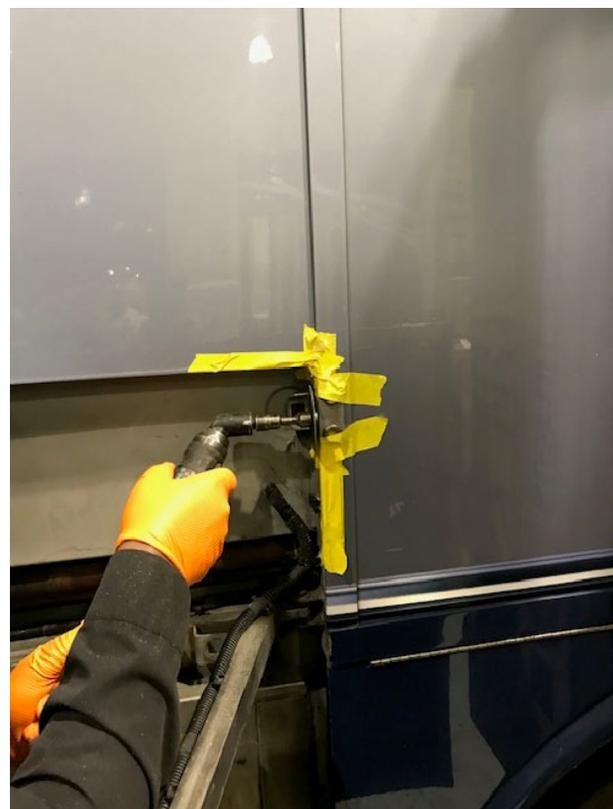
25. Drill two pilot holes on the door frame using the **36381** jig as a guide as shown.
