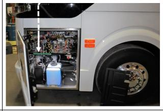
13. Connect the ring terminal of the wire to one of the front junction box ground studs.
