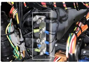
14. Reconnect A139 and A103 connectors and power-on the vehicle to confirm that all the steering wheel buttons are working properly.
