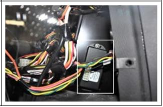
7. Using extractor tool **681485**, remove the terminals located at PIN 2 (A55RJ1.18 wire) from the <u>A139</u> module connector.
