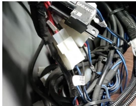
30. Plug the left harness with the short side of the power harness and route the extra cable around the electrical center.
