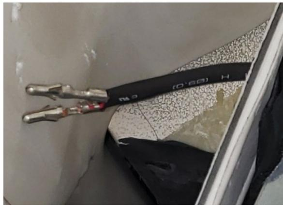
12. Install the harness on the sensor.
