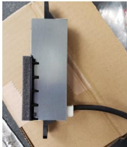
13. Install the isolation supplied with the sensor, around the harness connection on the sensor.
