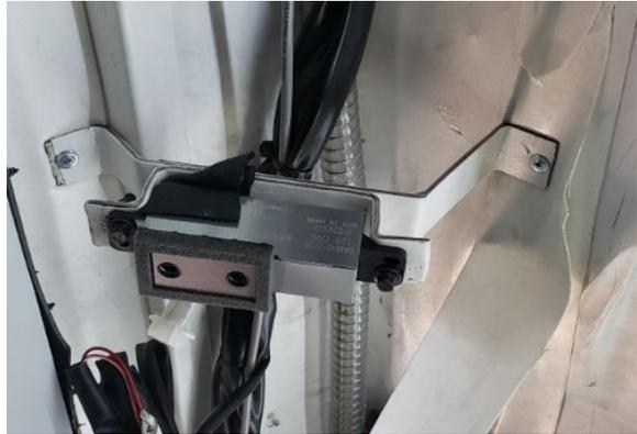
17. Route the side harnesses 24162221 inside the duct. Fix it with cable ties.
