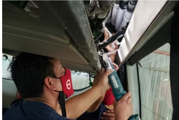
11. Join the black cables, crimp a 968016 terminal on the black and red cables.
