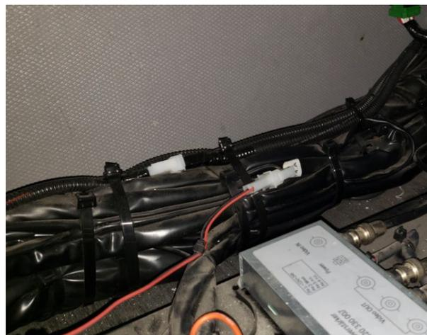
31. Cross the remaining harness under the stairs to the front electrical compartment on the right side.
