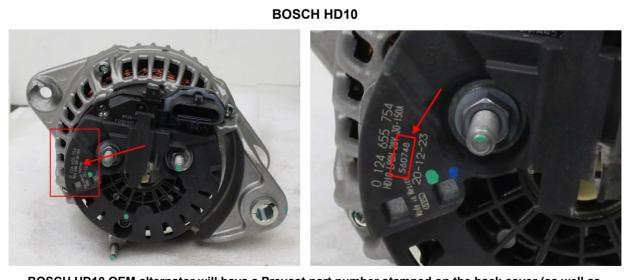
BOSCH HD10 OEM alternator will hava a Prevost part number stamped on the back cover (as well as Bosch part numbers). <image><section-header>
