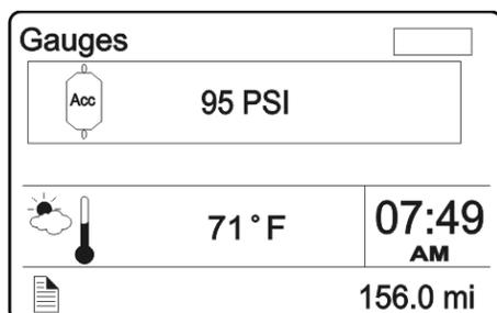
FIGURE 3: ACCESSORY PRESSURE GAUGE IN DRIVER INFORMATION DISPLAY
