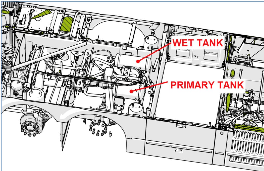
FIGURE 1: AIR TANKS LOCATION (LATEST ARRANGEMENT) – REAR END
