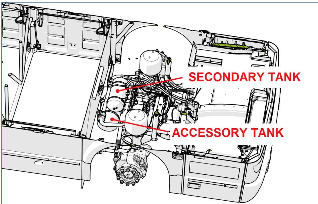
FIGURE 2: AIR TANKS LOCATION (LATEST ARRANGEMENT) – FRONT END
