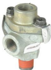
The double check valve is located on the pneumatic accessories panel in the front service compartment. In the event of a pressure drop in either the primary or secondary system, this unit will protect the emergency /parking brake control valve and the intact portion of the air system from pressure loss.
