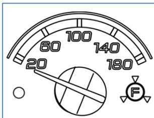
FIGURE 4: SECONDARY SYSTEM AIR PRESSURE GAUGE – FRONT BRAKES
