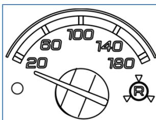
FIGURE 5: PRIMARY SYSTEM AIR PRESSURE GAUGE – REAR BRAKES
