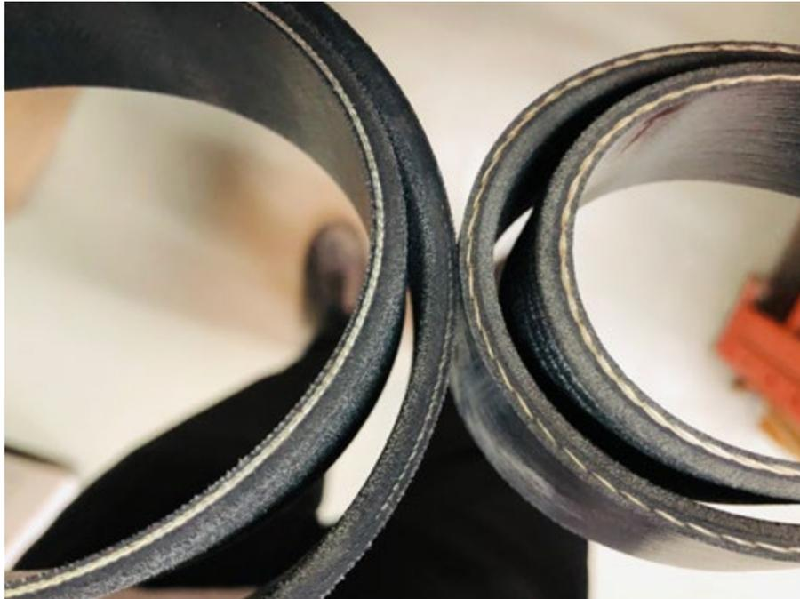
Defective Aramid cord reinforced belt (left) vs New polyester cord belt (right)
