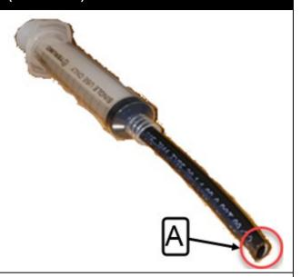
3. Fill the syringe with glue 684743 using gun (pneumatic or manual).
