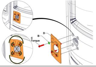
3. Plug connector (B) to the left mirror (A). 4. Install left mirror (C) 1. Tilt mirror towards vehicle. 2. Press down on top of anchor plate. 3. Lower it into place. 5. Install Bolt (D) with a torque 72lb-in. D Torque
