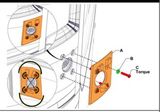
2. Install right anchor plate (D) with washer (B) 5001341 (4x) and bolt (C) 5002142 (4x) with a torque 14 lb-ft.
