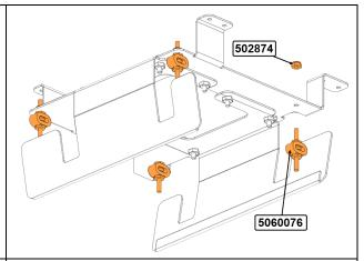
7. Install the subwoofer 901193 on the mount with flat washers 500577 (4x) and nuts 502874 (4x). Make sure the speaker connector is positioned as shown.
