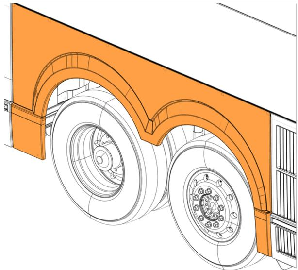
2. Clean the structure supporting the mudguard.
