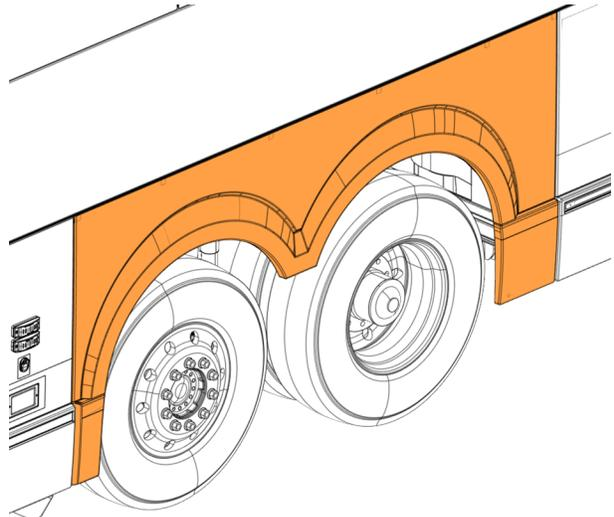
2. Clean the structure supporting the mudguard.
