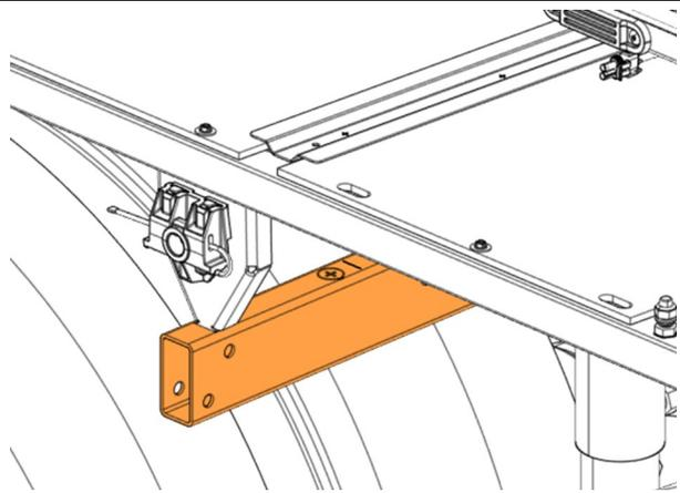
3. Secure the mudguard 460565P with screws 5001185(4x), washers 500270(8x) and nuts 5001787(4x).
