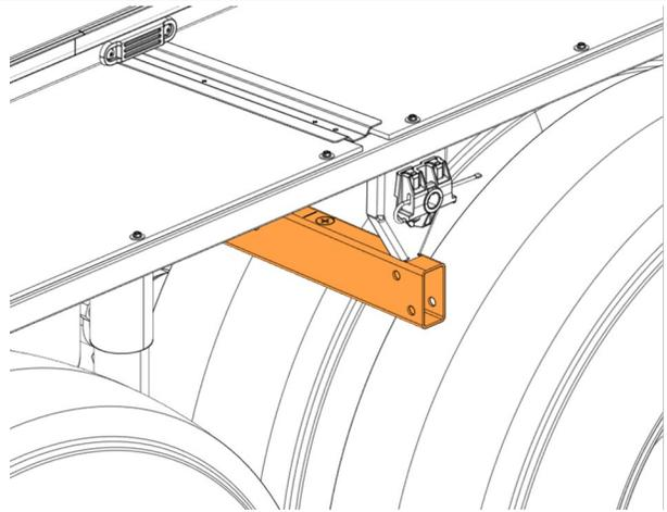
3. Secure the mudguard 460566P with screws 5001185(4x), washers 500270(8x) and nuts 5001787(4x).
