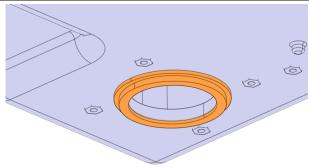
11. Add a Ø1/8" bead of Simson glue (684685) around the gasket. **Do not spread with your finger.**
