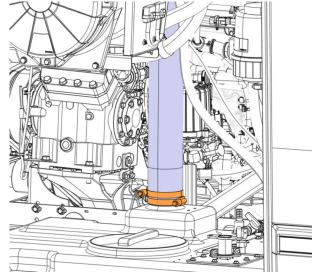
2. Ensure that the existing reinforcing sleeve on the main tank is still in place.
