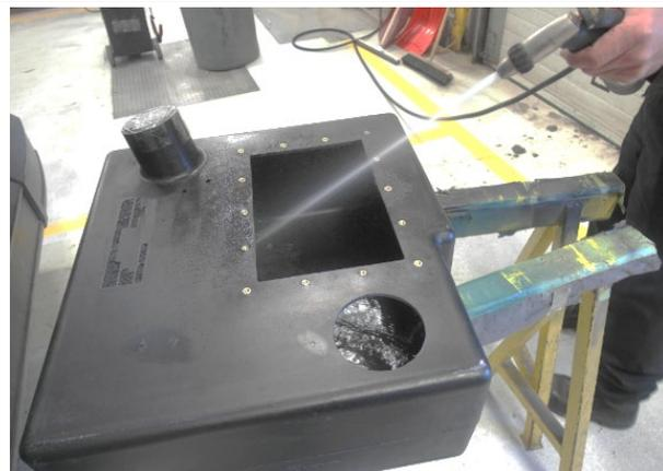
20. Install the assembled trap 404176 inside the tank with the gasket 404155, bolts 502737 (2x), flat washers 500411 (2x) and nuts 5001182 (2x).
