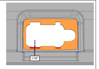
9. Install catch 313667 with screws 500638 (2x) and washers 500855 (2x), use same hole than older catch.
