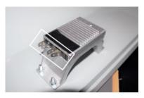
Remove the four screws (two at each end) holding the blower assembly to the AC unit.
