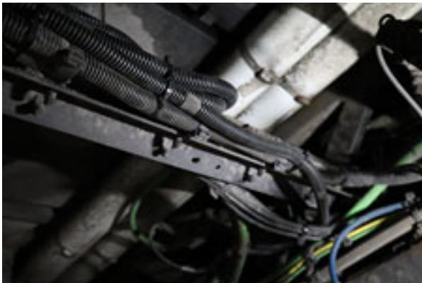
3. Seal the hole between baggage compartment and rear axle compartment with 684517.
