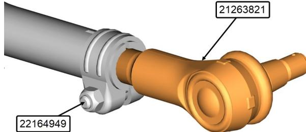
5. Adjust the drag link to the correct length 70mm (A) and fit it to the Pitman arm, checking that the steering gear is in the centre position. If not, adjust the drag link.
