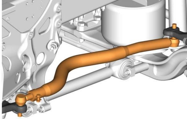
3. Remove castle nut and split pin the drag link from the steering arm and discard.
