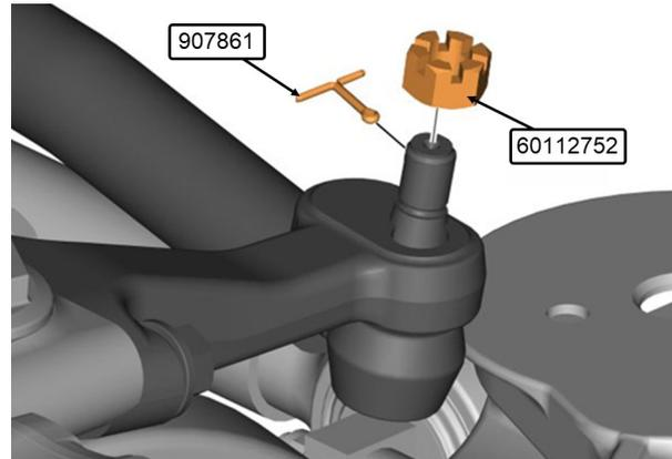
12. Adjust the drag link to the correct length 70mm (A) and fit it to the Pitman arm, checking that the steering gear is in the centre position. If not, adjust the drag link.
