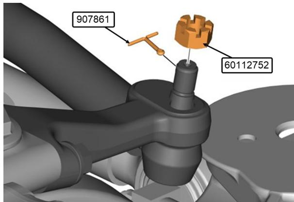
10. Disassembly the drag link from the pitman arm and discard the split pin.
