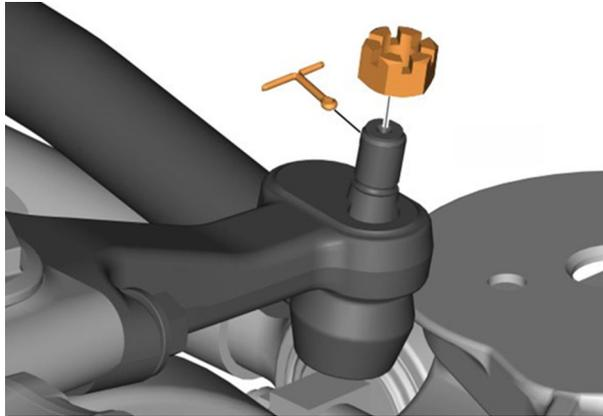
4. Disassembly the drag link from the steering arm with tool 9990814.
