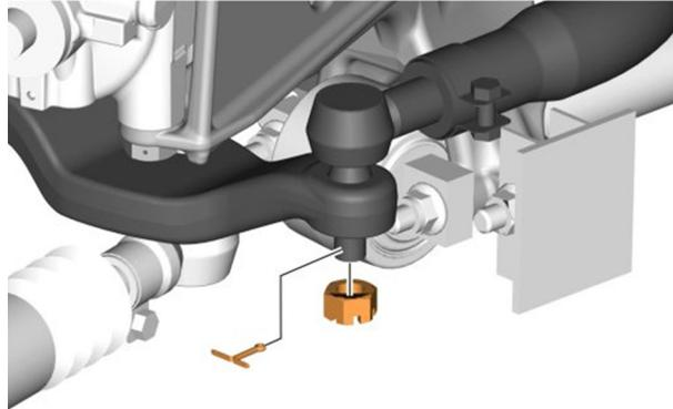
6. Disassembly the drag link from the pitman arm with tool 9990814.
