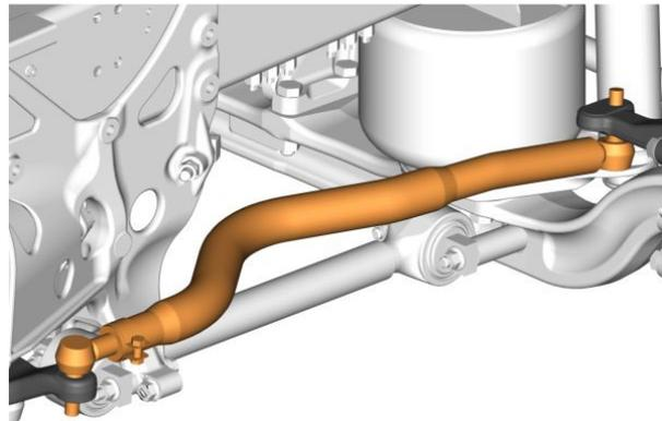
9. Install a new castle nut 60112752 on the drag link from the steering arm.
