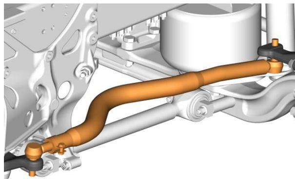
4. Disassembly the drag link from the steering arm and discard the split pin.
