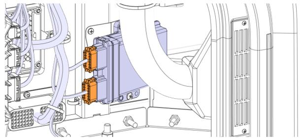
3. Unscrew the two (2) screws that hold the old module.
