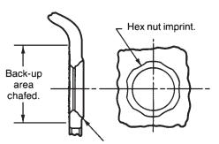
Chamfer enlarged or wallowed out by nut. Causes: Loose cap nuts or insufficient nut torque due to damaged threads, improper torquing or by wornout nut.
