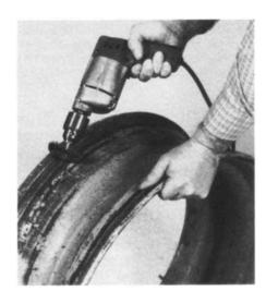
Bead seat areas of rim should be free of rust and rubber deposits. This is especially important for drop-center tubeless rims, because the bead seat is the air-sealing element.
