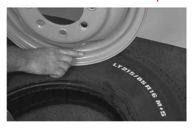
WARNING: Mounting a smaller diameter tire on a larger diameter rim/wheel (for example, a 16-inch tire on a 16.5-inch rim/wheel) can result in failure of the tire bead during mounting or airing. Mounting a larger diameter tire on a smaller diameter rim can result in unseating of the tire bead during operation. The tire may explode, striking a worker or bystander with deadly force. Check tire and rim/wheel diameter before starting to mount the assembly.
