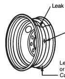
Leak at butt weld. Cause: Overload.
