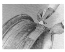
Paint rim by brush or spray with a fast-drying metal primer. Surfaces should be clean and dry prior to painting. Ensure that bare metal areas on outside or tire side of rim are covered. This is especially important on drop-center tubeless rims, because warm and sometimes moist air is in constant contact with the metal surface on the tire side of the rim.
