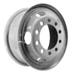
**Tube-Type Disc Wheel Assembly**
