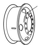
Cracks at disc nave and/or handhole. Causes: Bad fit-up, damaged hub, overload or sharp edge at handhole.
