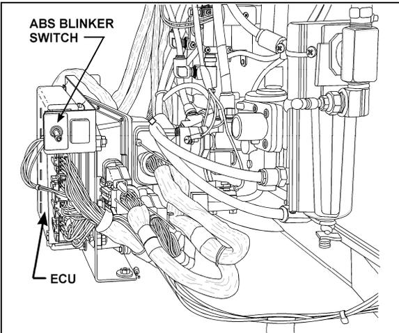
FIGURE 23: BOTTOM SECTION OF FRONT SERVICE COMPARTMENT 06394
