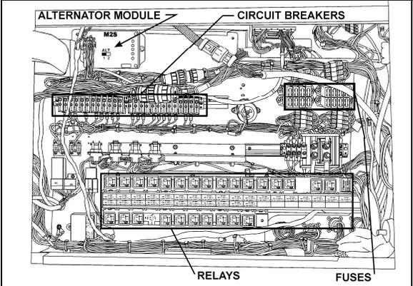
FIGURE 22: TOP SECTION OF FRONT SERVICE COMPARTMENT 06319
