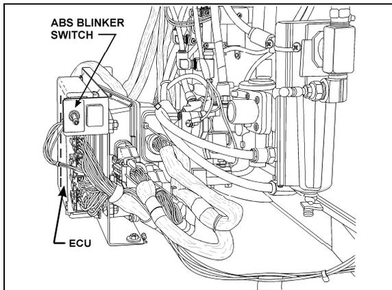
FIGURE 10: BOTTOM SECTION OF FRONT SERVICE COMPARTMENT
