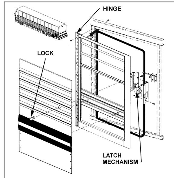
FIGURE 47: L.H. SIDE REAR SERVICE COMPARTMENT DOOR
