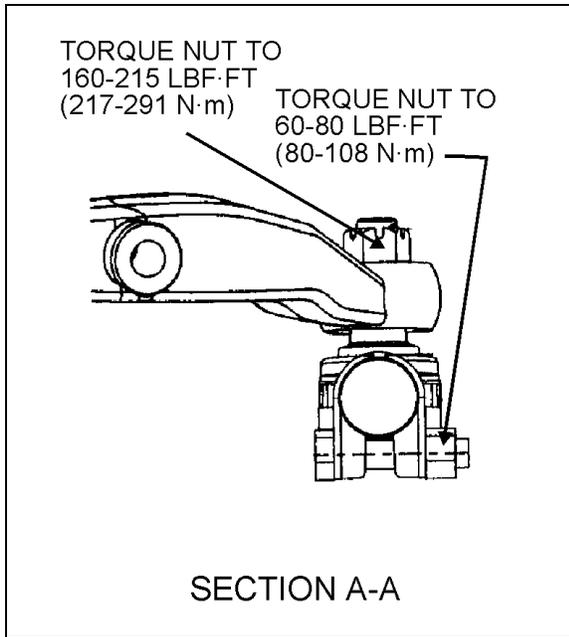
FIGURE 3: CLAMP POSITIONING
