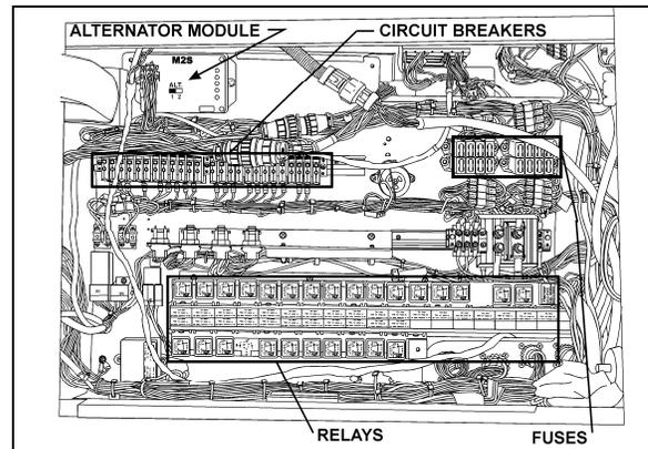
FIGURE 9: TOP SECTION OF FRONT SERVICE COMPARTMENT
