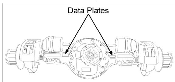
FIGURE 1: TYPICAL SERIAL & MODEL NUMBERS 11019
