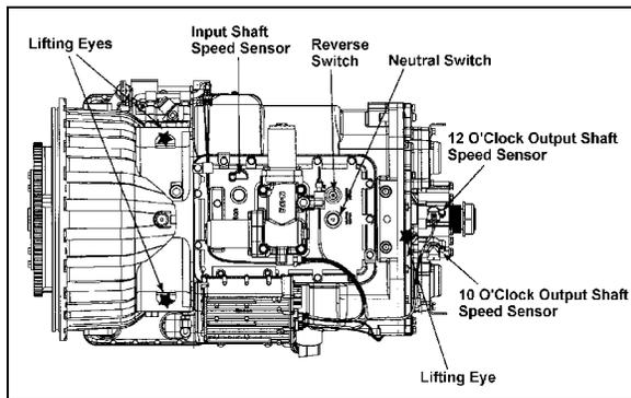
FIGURE 21: LIFTING EYES AND SENSOR POSITION<sup>07068</sup>
