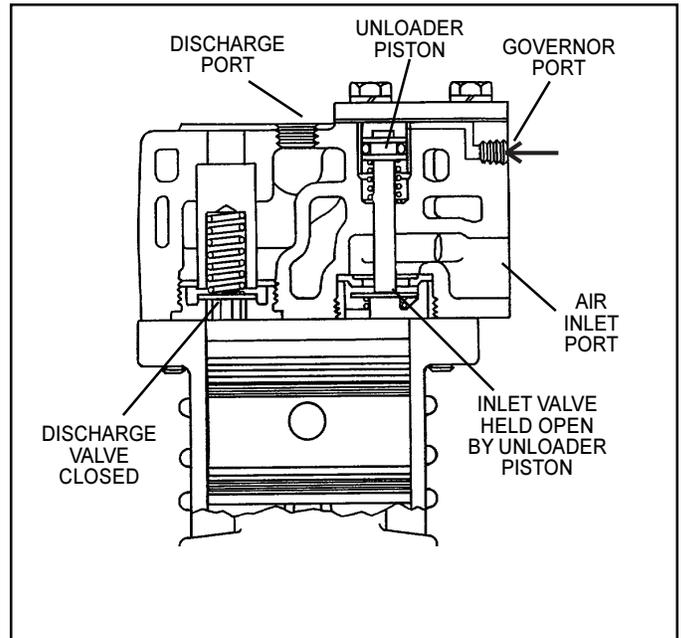
FIGURE 6 - OPERATIONAL-UNLOADED
