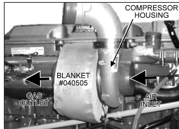
FIGURE 6: TURBO BLANKET INSTALLATION
