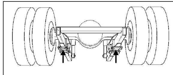
FIGURE 53: JACKING POINTS ON DRIVE AXLE
