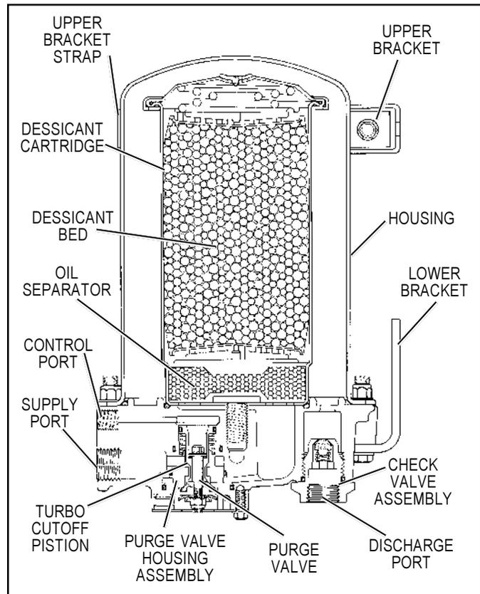
FIGURE 5 - AD-9 AIR DRYER SECTIONAL VIEW
