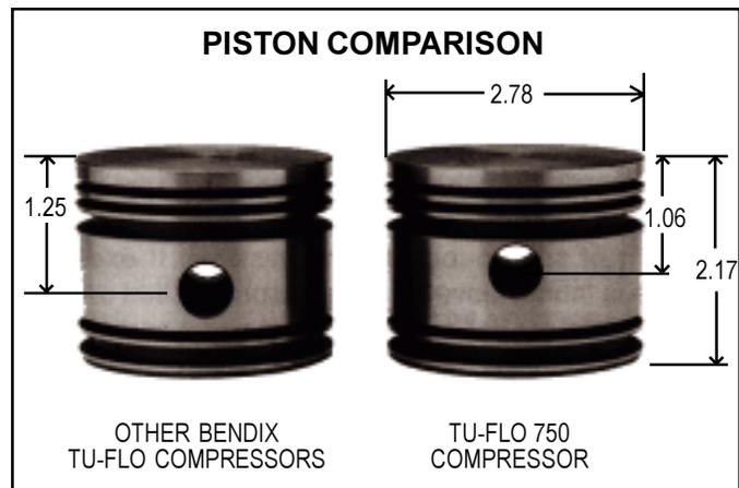
FIGURE 13 - PISTON COMPARISON
