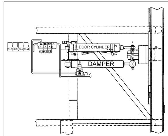
FIGURE 17: DOOR CYLINDER AND DAMPER
