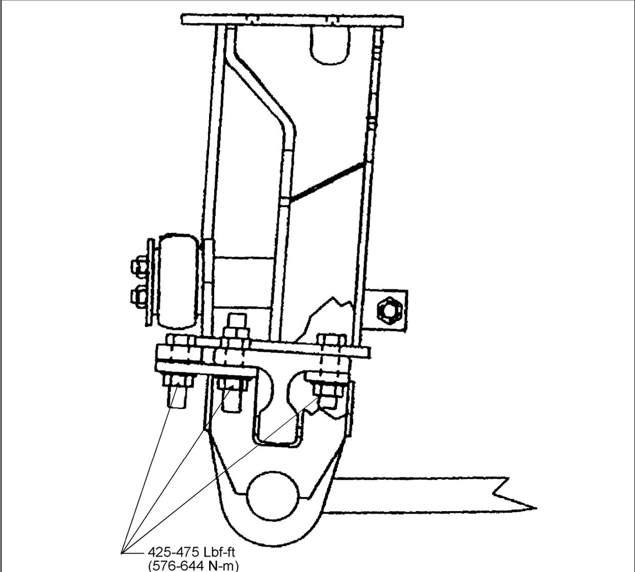
FIGURE 6: AIR BELLOWS MOUNTING SUPPORT AND AXLE
