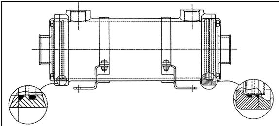
FIGURE 19: OIL COOLER INSTALLATION
