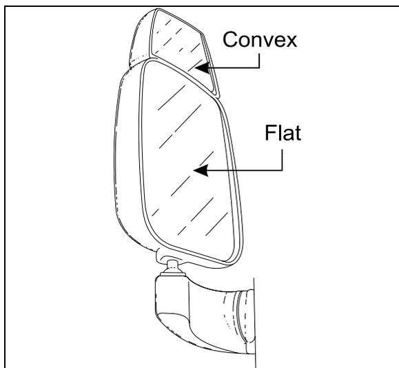
FIGURE 49: REAR VIEW MIRROR (RAMCO) 18398A
