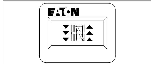
**FIGURE 3: GEAR DISPLAY MODULE** 07056
