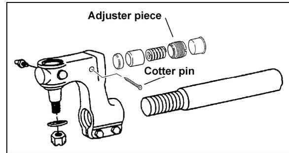
FIGURE 2: TIE ROD END PLAY ADJUSTMENT
