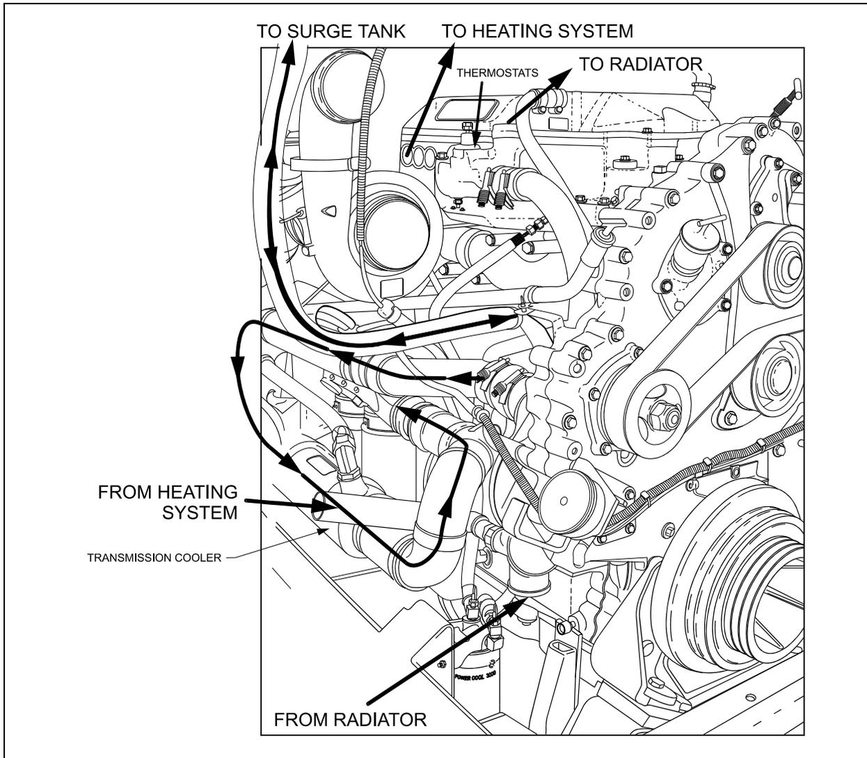
FIGURE 1: COOLING SYSTEM
