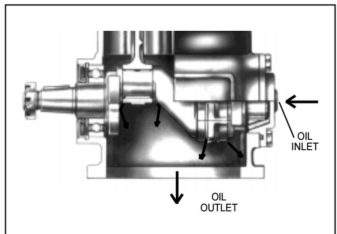
FIGURE 7 - LUBRICATION (BASE MOUNT MODEL SHOWN)
