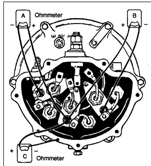
FIGURE 37: STATOR WINDING TEST
