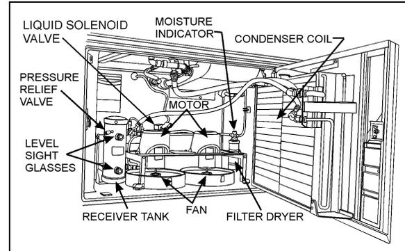
FIGURE 28: A/C CONDENSER COMPARTMENT 22174
