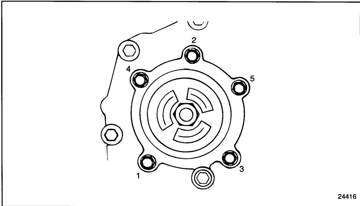
**Figure 1-413 Accessory Drive Housing Bolt Torque Sequence**
