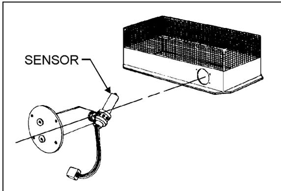
FIGURE 6: THERMISTOR SENSOR 22064
