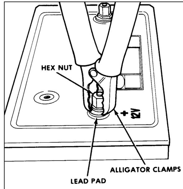
FIGURE 30: ALLIGATOR CLAMPS AND BATTERY 06065
