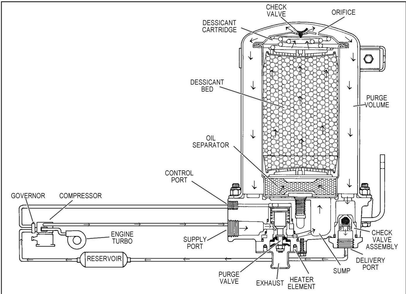
FIGURE 2 - AD-9 CHARGE CYCLE
