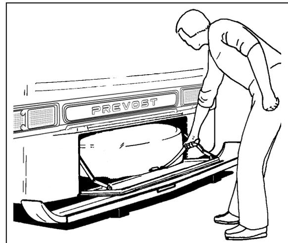
**FIGURE 8: REMOVING SPARE WHEEL AND TIRE**
