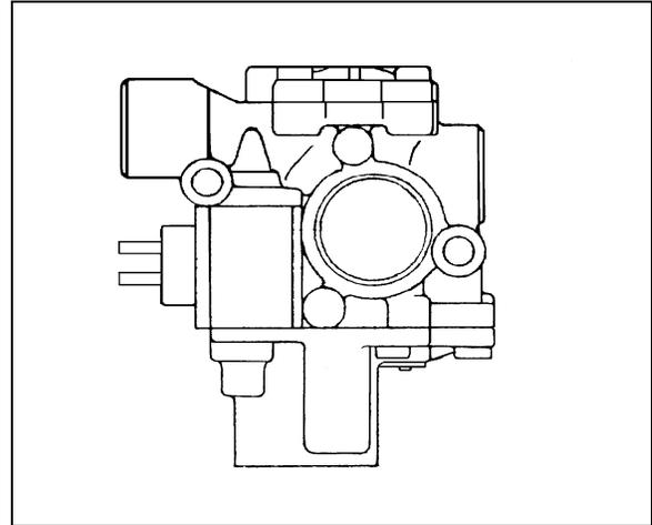
FIGURE 45: ABS MODULATOR VALVE 12084
