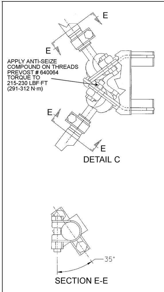
FIGURE 6: CLAMP POSITIONING
