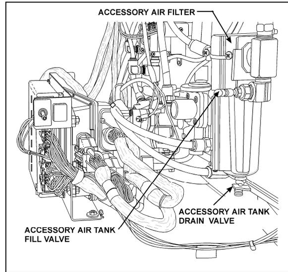
FIGURE 29: FRONT VALVE LOCATION
