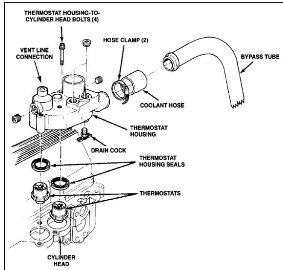
FIGURE 12: THERMOSTAT AND RELATED PARTS 05034
