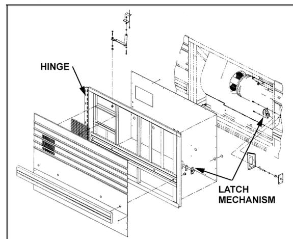
FIGURE 45: EVAPORATOR DOOR
