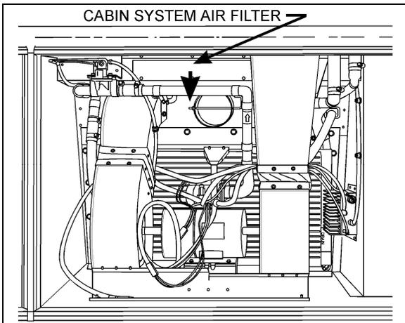
FIGURE 14: CABIN SYSTEM AIR FILTER REMOVAL 22178
