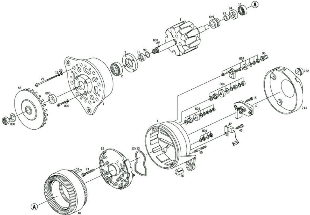
**Figure 4 Alternator Exploded View**
