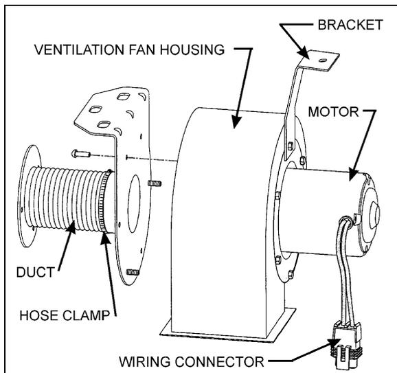
FIGURE 23: VENTILATION FAN INSTALLATION 23222
