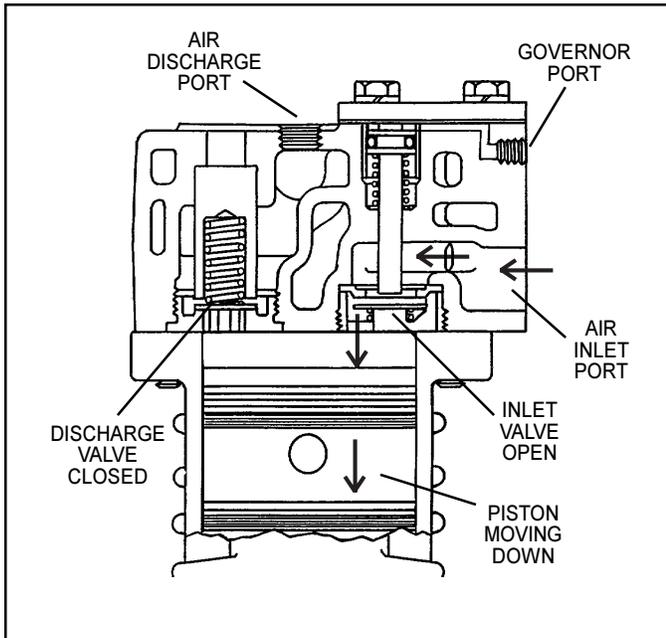
FIGURE 4 - OPERATIONAL-LOADED (INTAKE)
