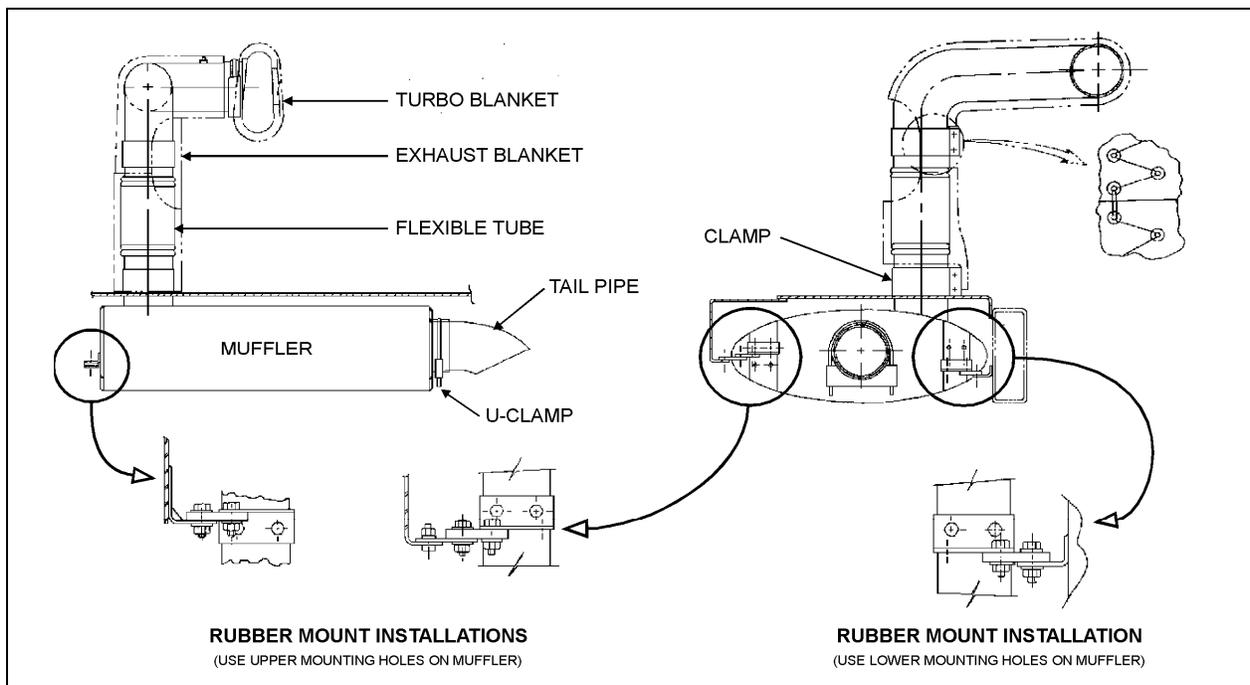
FIGURE 1: EXHAUST SYSTEM - XL2-40 & 45E (COACH & SHELL) INSTALLATION
