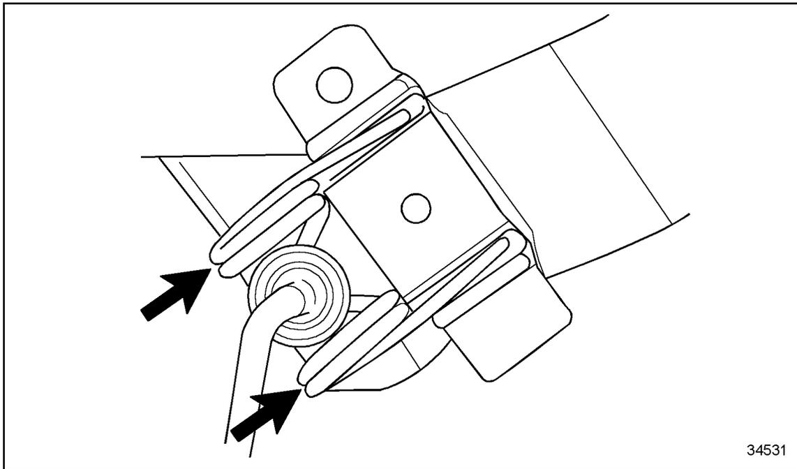
**Figure 1-434**      **Installing the Slave Piston Assembly Torsion Spring**
