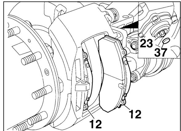
FIGURE 35: PAD INSTALLATION 12111
