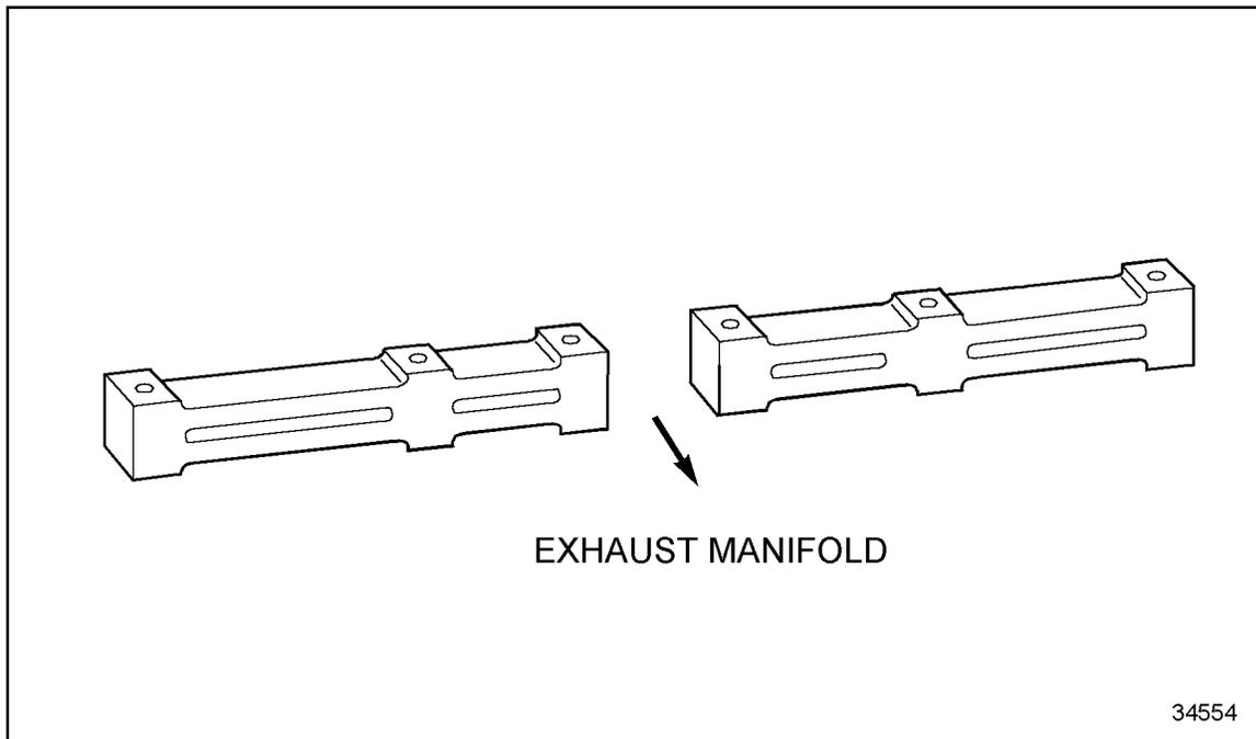
**Figure 1-435**      **Spacer Bars with "Out" Marks Adjoined**
