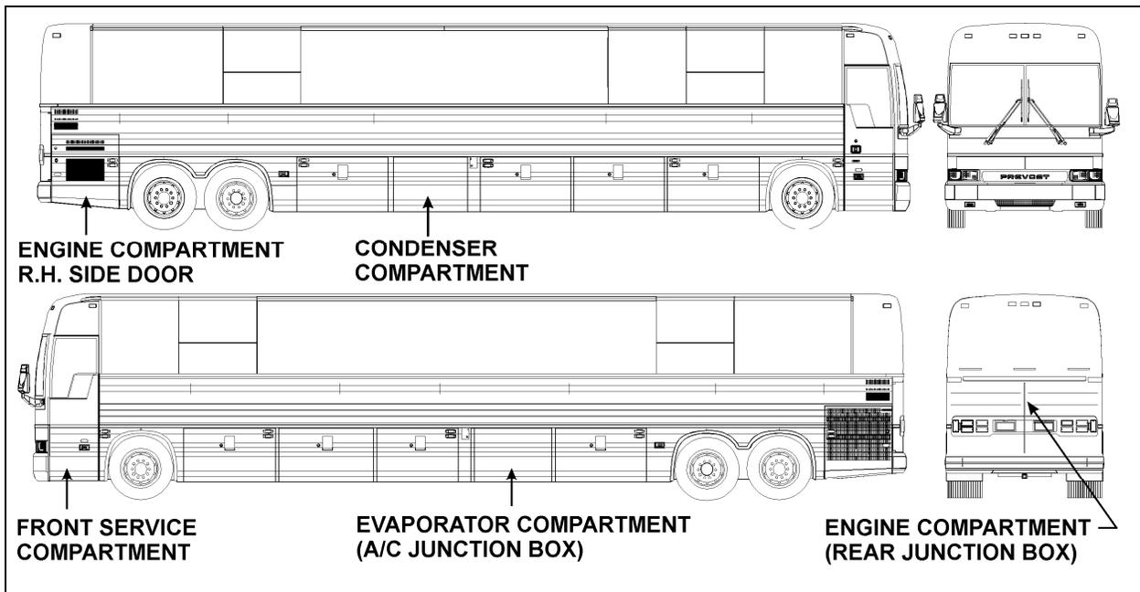
FIGURE 16: ELECTRICAL COMPARTMENTS (XL2-45E BUS SHELLS)
