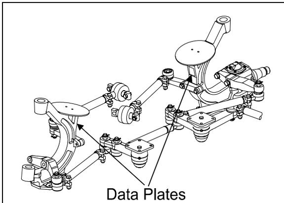
FIGURE 6: ISS TYPICAL SERIAL & MODEL NUMBERS
