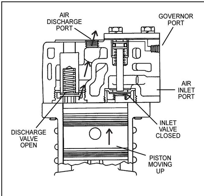
FIGURE 5 - OPERATIONAL-LOADED (COMPRESSION)
