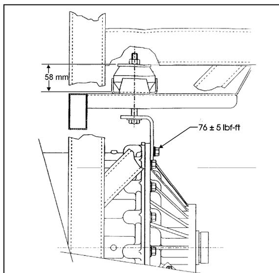
FIGURE 22: NUT TOLERANCE
