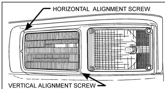
FIGURE 58: ALIGNMENT SCREWS
