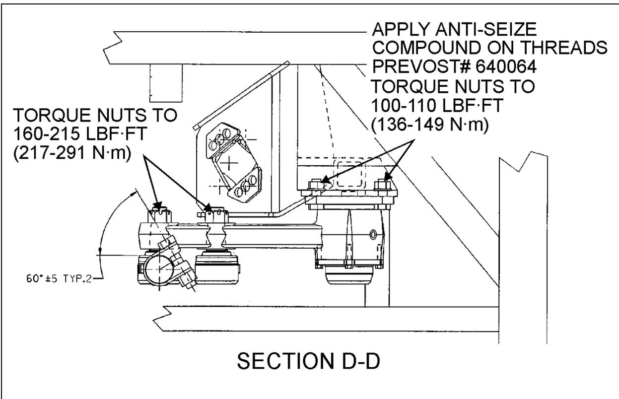
FIGURE 5: CLAMP POSITIONING
