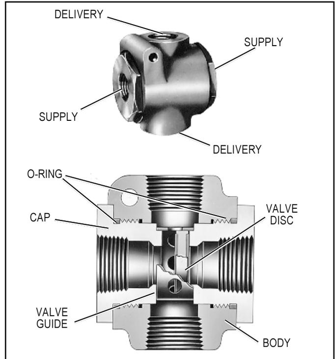
FIGURE 2 - DOUBLE CHECK VALVE (DISC TYPE)
