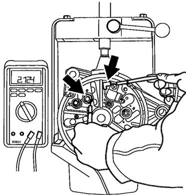
**Figure 8 Testing of Suppression Capacitor**
