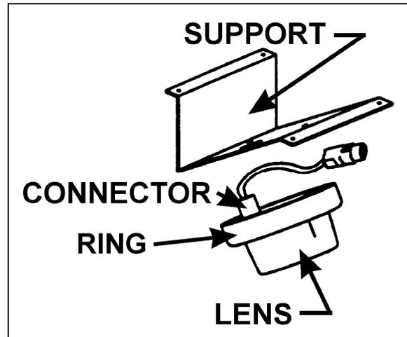
FIGURE 63: ENGINE COMPARTMENT LIGHT
