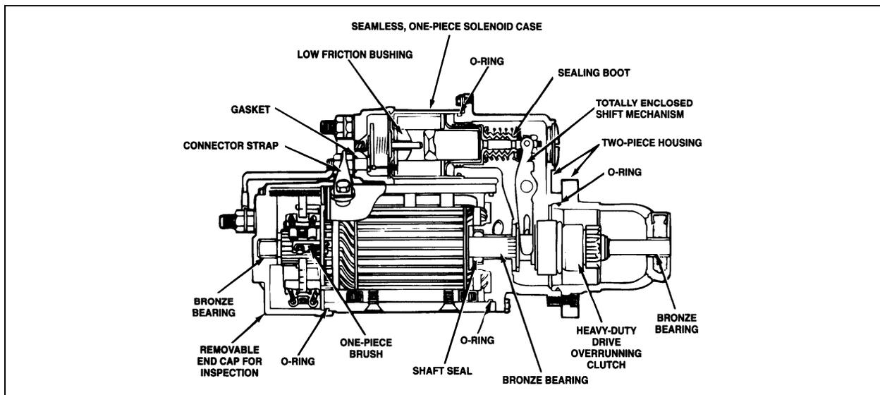
FIGURE 48: TYPICAL STARTER CROSS SECTION
