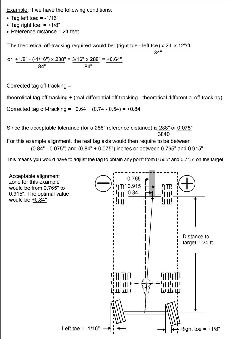
**FIGURE 10: EXAMPLE CALCULATION**
