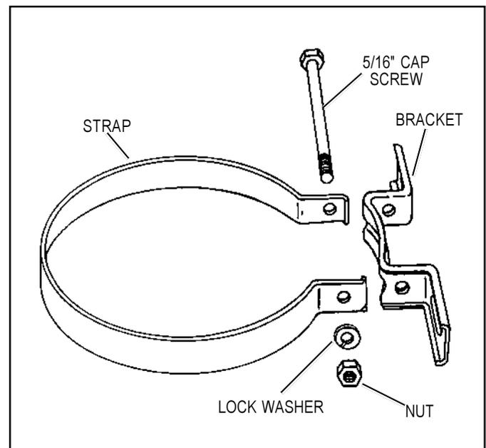
FIGURE 10 - UPPER MOUNTING BRACKET AND STRAP
