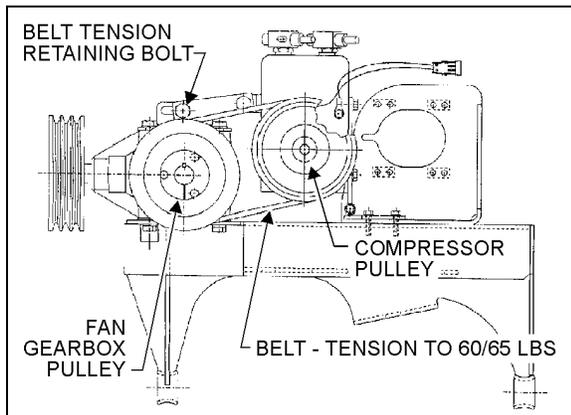
**FIGURE 26: A/C COMPRESSOR (DRIVER'S OR AUXILIARY SYSTEM)**
