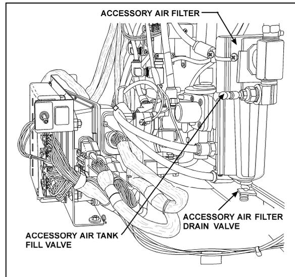
FIGURE 3: FRONT SERVICE COMPARTMENT 12144
