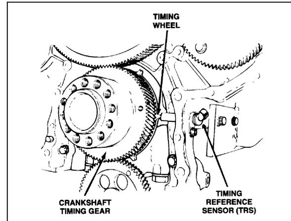
FIGURE 6: TIMING GEAR
