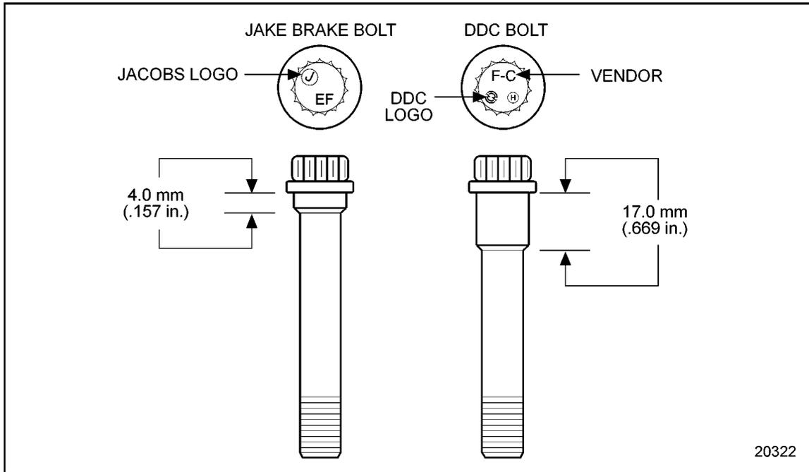
**Figure 1-437 Jake Brake and DDC Bolt Identification**
