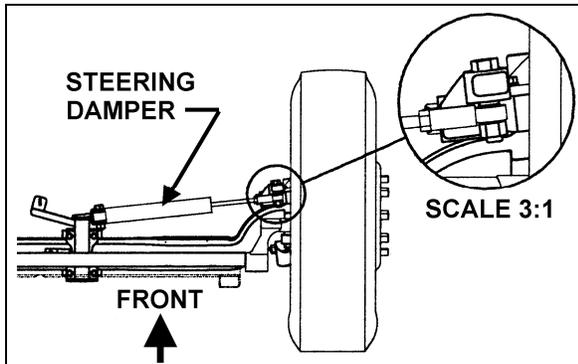
FIGURE 9: STEERING STABILIZER (DAMPER)
