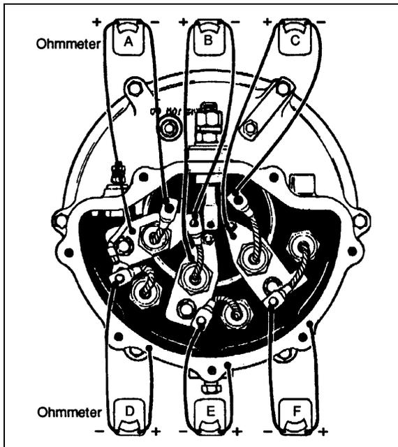
FIGURE 36: DIODE TESTING
