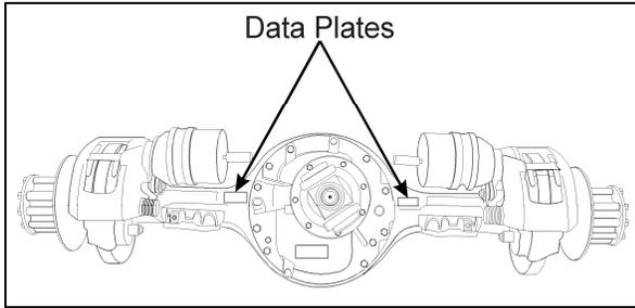
FIGURE 4: TYPICAL SERIAL & MODEL NUMBERS 11019
