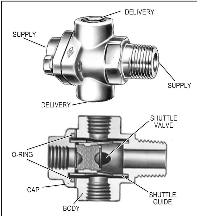
FIGURE 1 - DOUBLE CHECK VALVE (SHUTTLE TYPE)
