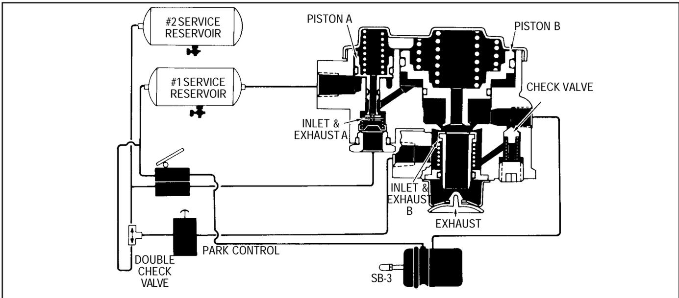
FIGURE 8 - SERVICE APPLICATION - LOSS OF #1 RESERVOIR
