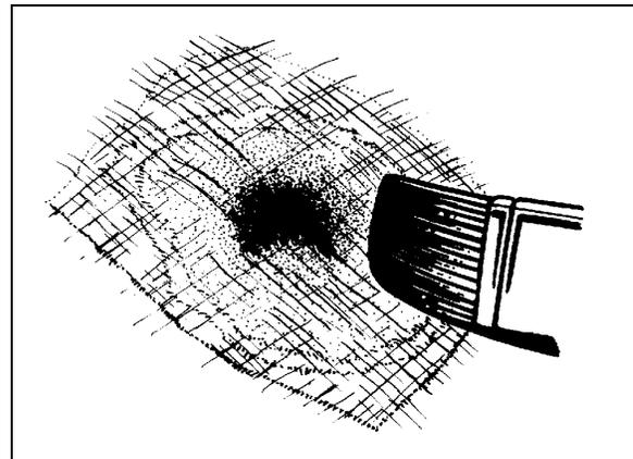
FIGURE 7: FIBERGLASS REPAIR
