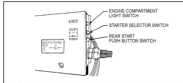
FIGURE 13: REAR JUNCTION BOX SWITCHES
