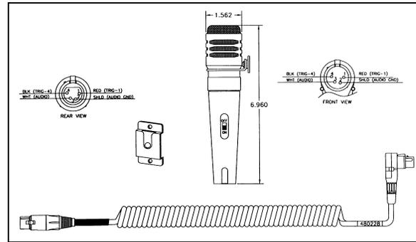
FIGURE 9: RUBBER COATED MICROPHONE 23217
