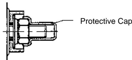
**Figure 31 Terminal W Insulator,
