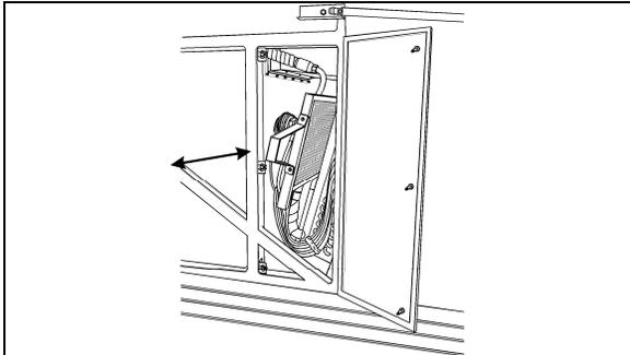
FIGURE 13: MAIN HVAC UNIT AIR FILTER 22179
