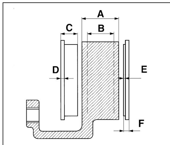
FIGURE 32: ROTOR AND PAD WEAR LIMITS 12113
