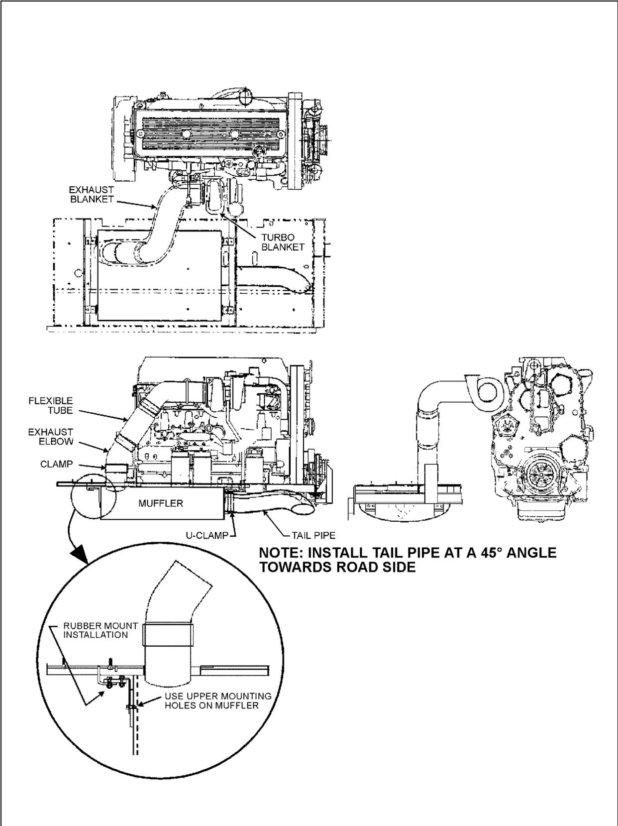
FIGURE 2: EXHAUST SYSTEM - XL2-45 (COACH & SHELL) INSTALLATION
