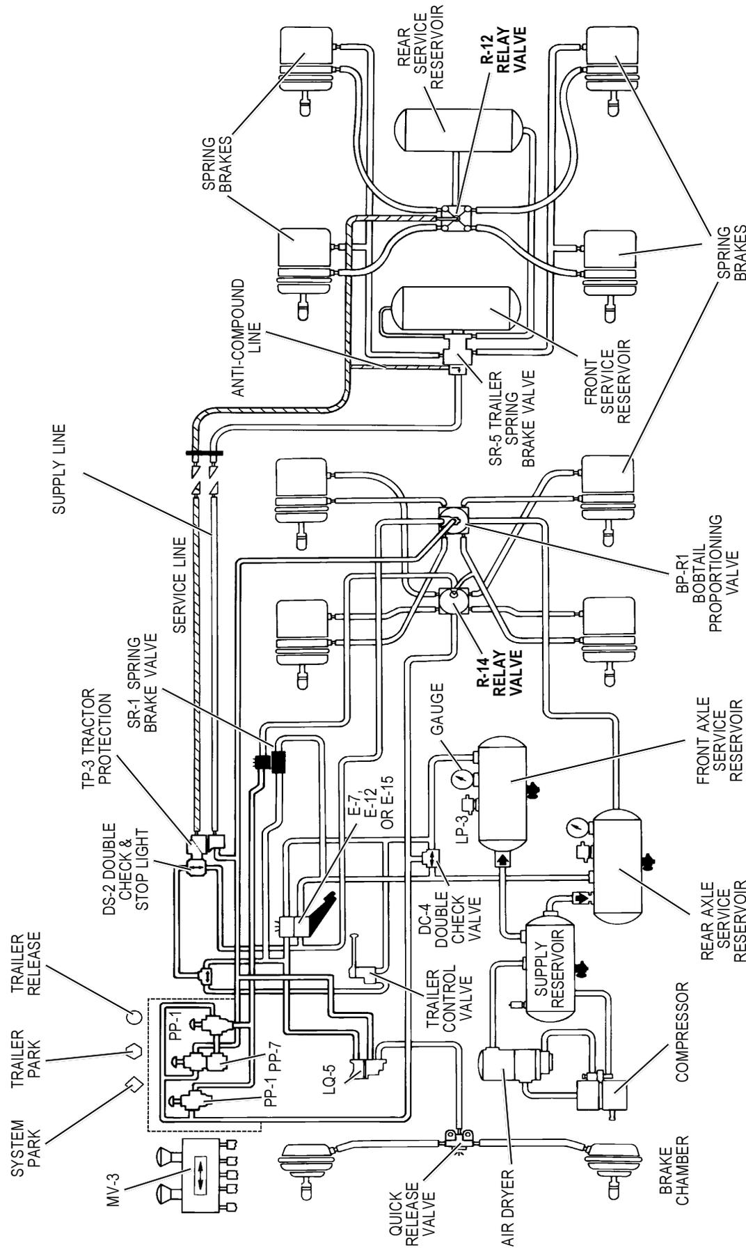
FIGURE 3 - TYPICAL PIPING SCHEMATIC
