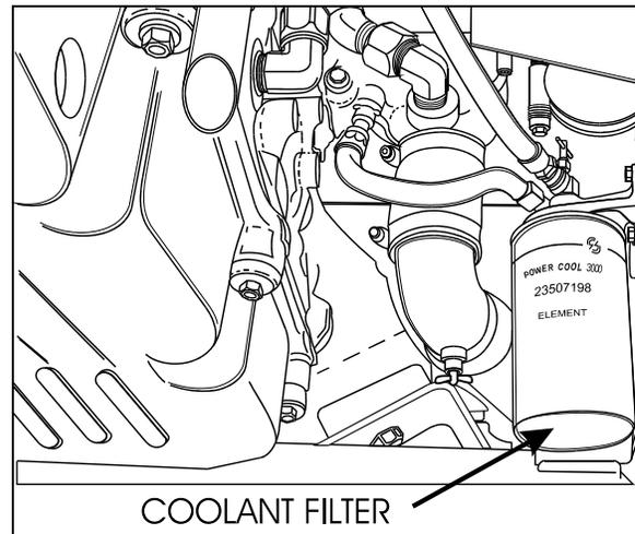
FIGURE 10: COOLANT FILTER
