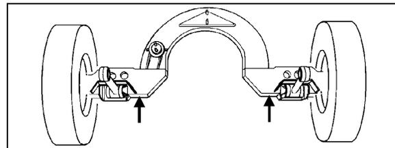
FIGURE 54: JACKING POINTS ON TAG AXLE
