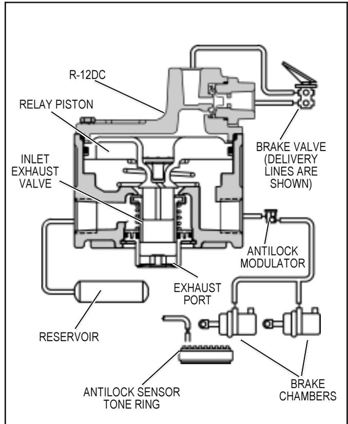
FIGURE 3 - R-12DC SECTIONAL VIEW WITH TYPICAL SYSTEM COMPONENTS
