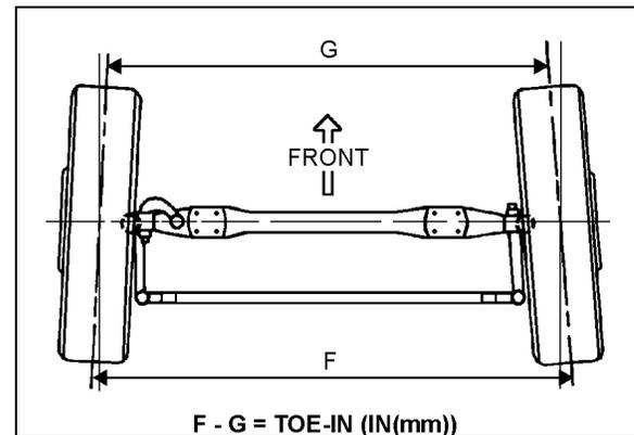
FIGURE 5: TOE-IN MEASUREMENTS
