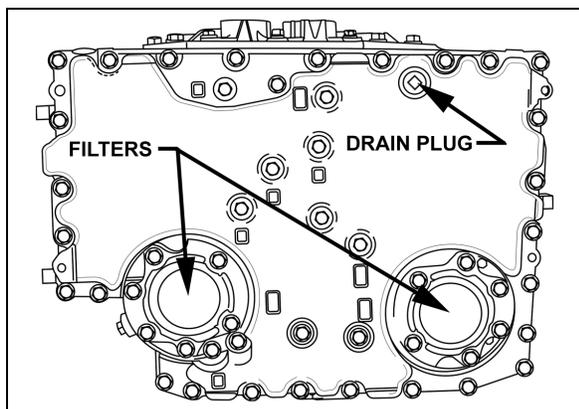
FIGURE 14: DRAIN PLUG AND FILTERS
