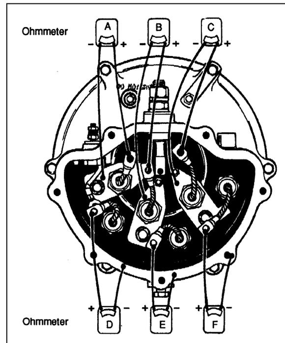
FIGURE 35: DIODE TESTING
