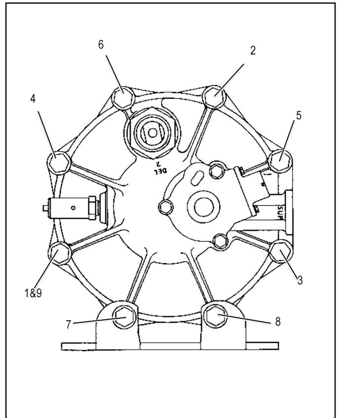
**FIGURE 8 - END COVER TO HOUSING TORQUE PATTERN INSTALLATION**
