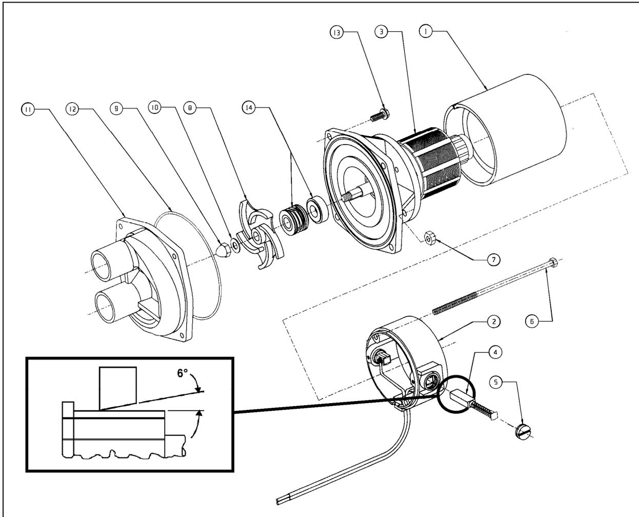
**FIGURE 48: WATER RECIRCULATING PUMP (CONVERTED VEHICLE - CENTRAL A/C)**
