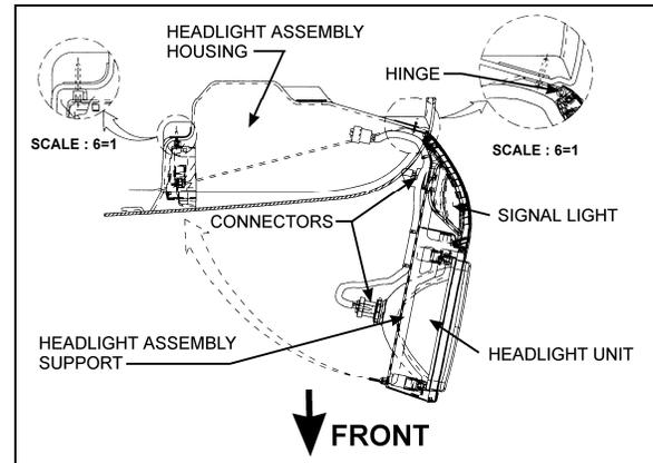
FIGURE 59: TOP VIEW OF HEADLIGHT ASSEMBLY
