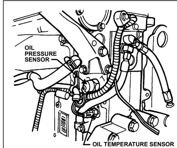
FIGURE 9: ENGINE OPS AND OTS
