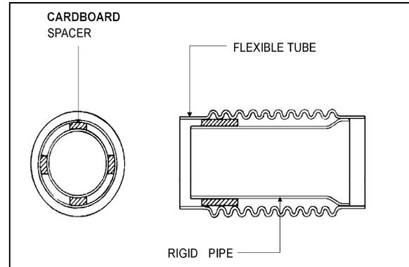
FIGURE 3: FLEXIBLE TUBE INSTALLATION 04003
