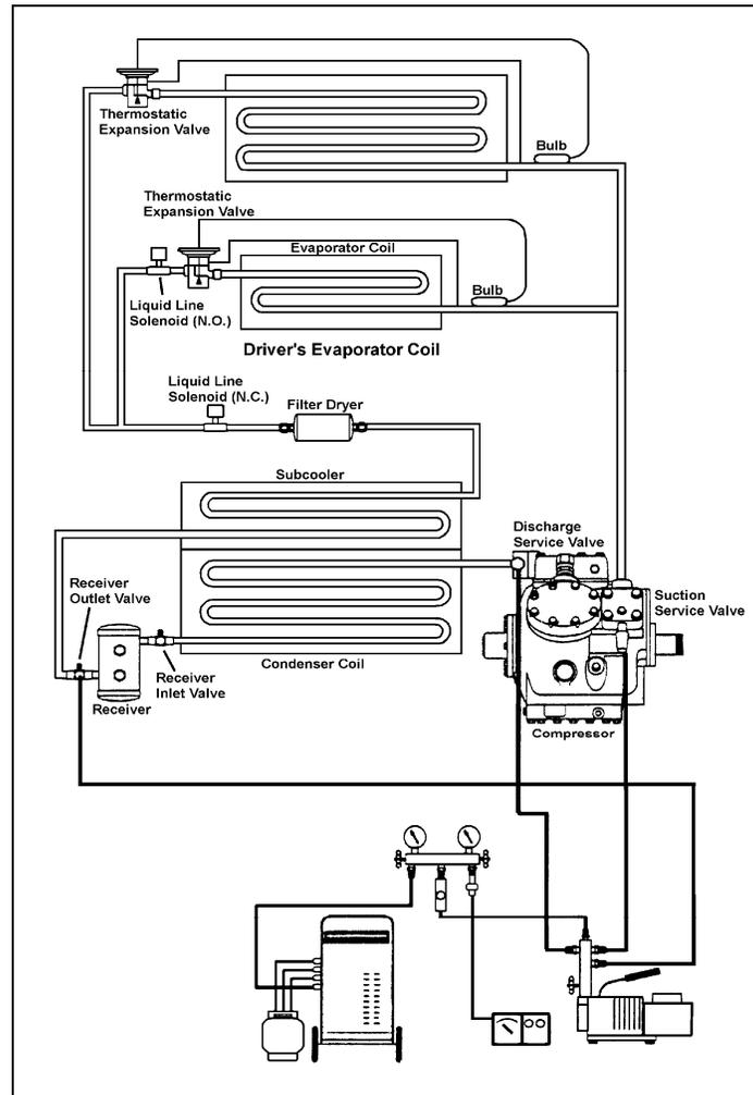
FIGURE 19: DOUBLE SWEEP EVACUATION SET-UP
