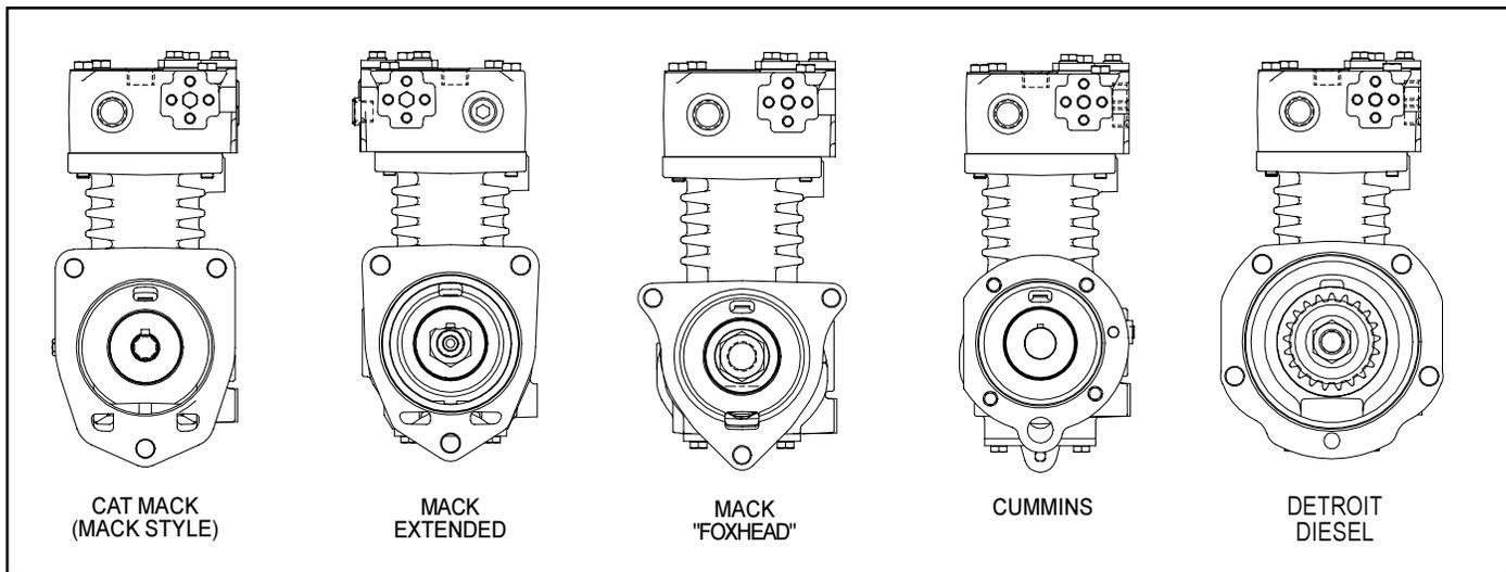
FIGURE 2 - MOUNTING CONFIGURATIONS
