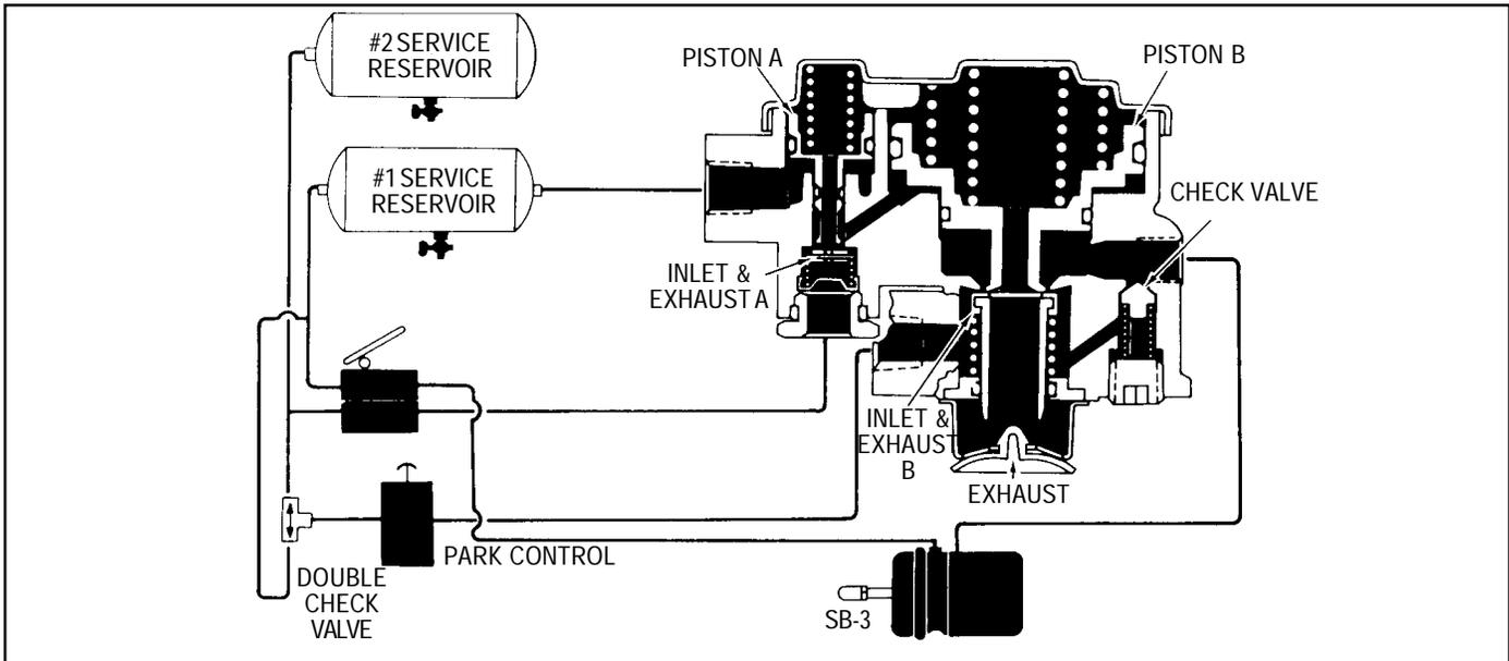
FIGURE 7 - SERVICE APPLICATION - LOSS OF #2 RESERVOIR
