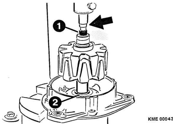
**Figure 28 Installing Rotor into Drive End Shield
