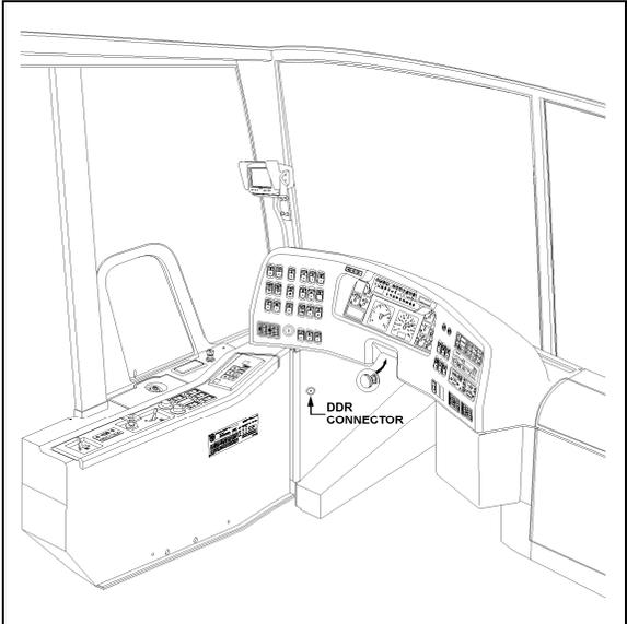
FIGURE 24: DDR CONNECTOR LOCATION IN DRIVER'S AREA 18375
