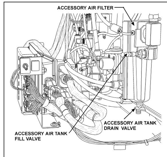
FIGURE 27: FRONT VALVE LOCATION
