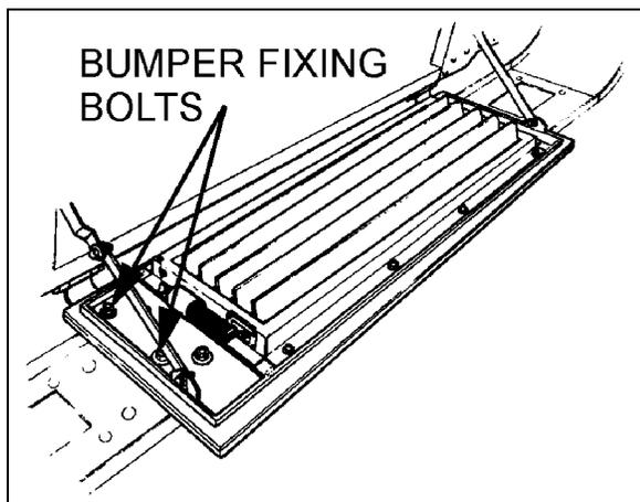
FIGURE 28: FRONT BUMPER REMOVAL
