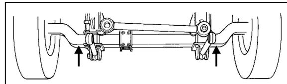
FIGURE 52: JACKING POINTS ON FRONT AXLE
