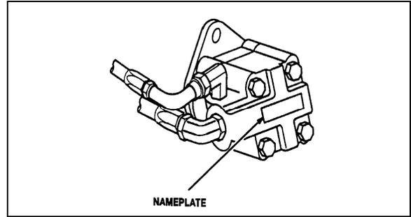
FIGURE 7 : POWER STEERING PUMP NAMEPLATE 00001
