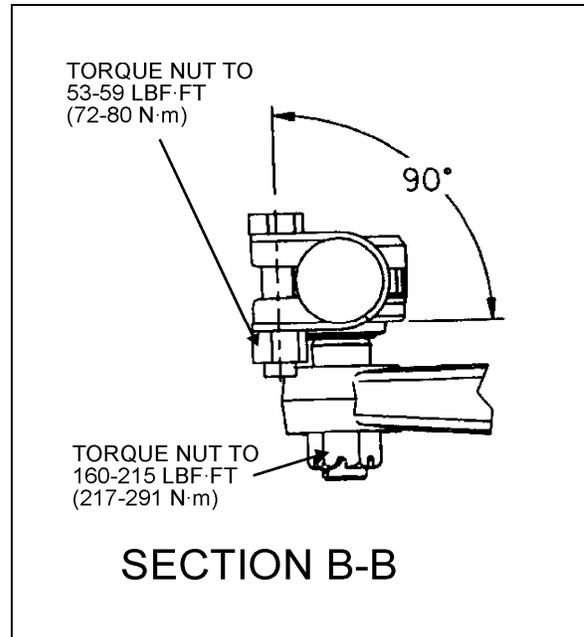
FIGURE 4: CLAMP POSITIONING
