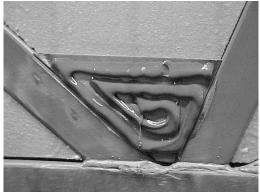
Apply glue beads onto the side panel. Do not forget to fill the first panel and last panel creases.
