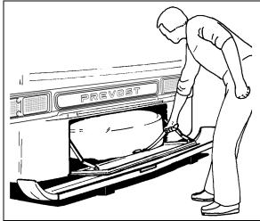
FIGURE 8: REMOVING SPARE WHEEL AND TIRE
